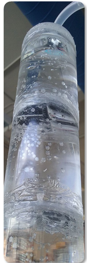
Figure 3.61. The build-up of bubbles seen during the long-term test of prototype #3
