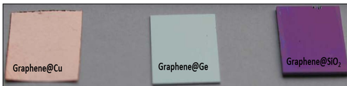
Figure 1.13 Copper (Graphene@Cu), Germanium (Graphene@Ge) and Silicon Dioxide (Graphene@SiO 2 ) substrates each coated with monolayers of graphene grown via CVD as reported by (Li et al. 2014).
