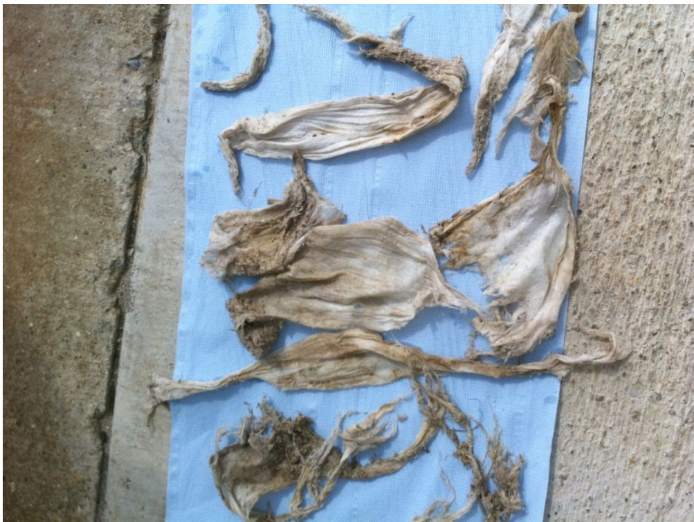
Figure 1-2 Samples of Blockage Material, Collected from Pumping Station
