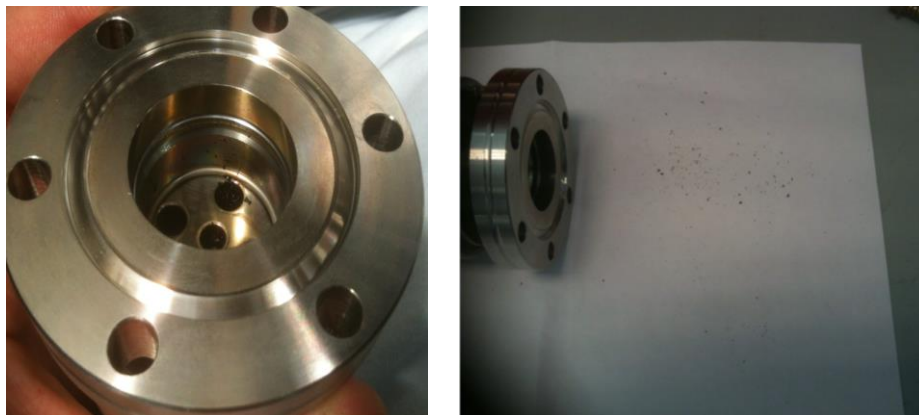
Figure A.8 Pictures of the contaminated gauge with the debris in the gauge (left) and debris made to fall on the paper (right) when gauge was tapped.
