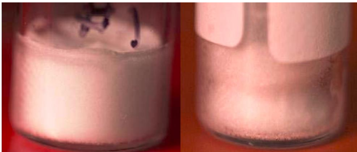
Figure 1-1: Comparison of an acceptable cake (left) and a collapsed cake (right) for an amorphous formulation. In the lower part of the collapsed cake a “ring” is observed indicating that this part of cake exceeded the collapse temperature and the amorphous material started to flow during primary drying
