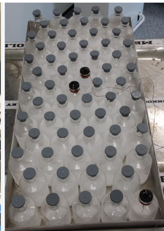
Figure 4-11: Vial configuration on the tray. TC were placed in the centre and front row of the tray
