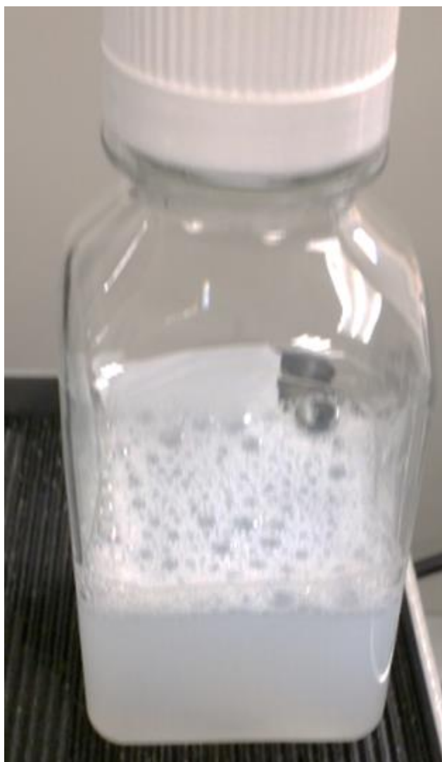
Figure 4-18: 120 g drug product. The formulation contained polysaccharide/Protein X conjugates, of serotype F and K along with other serotypes. Serotype F and K test articles lyophilised above and below collapse were individually formulated and the impact of polysaccharide biological function was assessed
