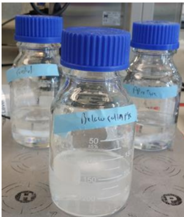
Figure 4-13: A 150 mL glass Duran vessel used for reconstitution. Each test article is reconstituted in solvent for a predefined time
