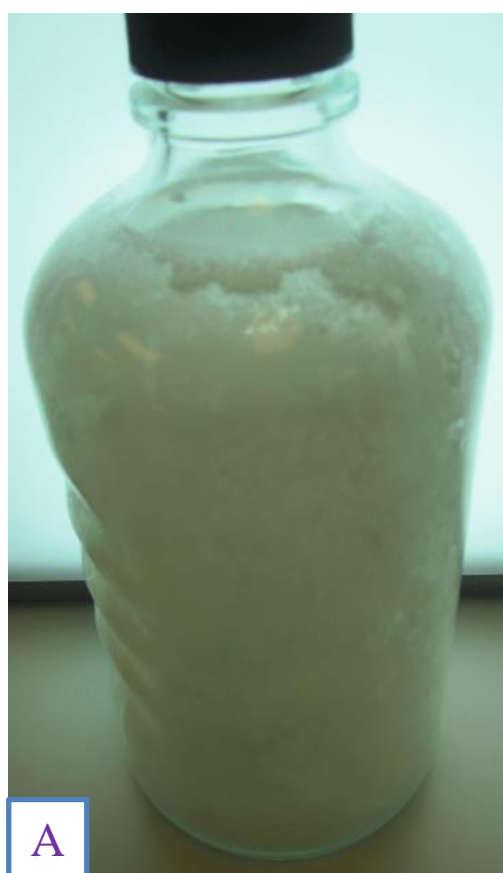
Figure 5-12: Serotype K control bottle, morphology rank 2 (A) and bottle freeze dried with 0.28 cm 2 aperture, morphology rank 4 (B)
