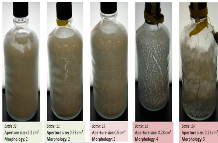
Figure 5-8: Influence aperture size on cake morphology
