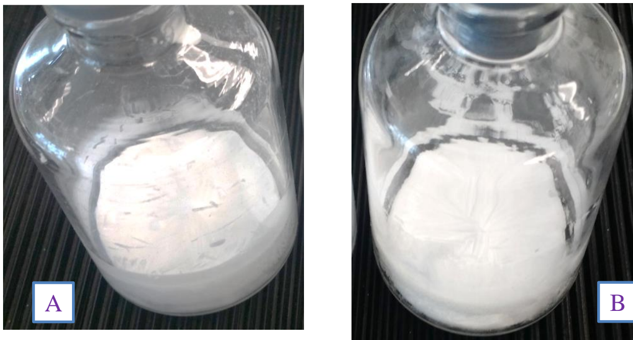
Figure 5-14: Cake appearance comparison serotype F freeze dried below collapse, (A) and freeze dried above collapse (B).
