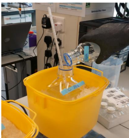
Figure 4-13: A 150 mL glass Duran vessel used for reconstitution. Each test article is reconstituted in solvent for a predefined time
