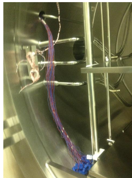
Figure 4-6: Feed-through is attached to blank port of dryer and TC fed into chamber.
