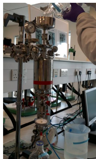
Figure 4-14: Transfer of reconstituted test article to a Chem glass reactor system for conjugation
