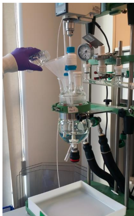
Figure 4-14: Transfer of reconstituted test article to a Chem glass reactor system for conjugation
