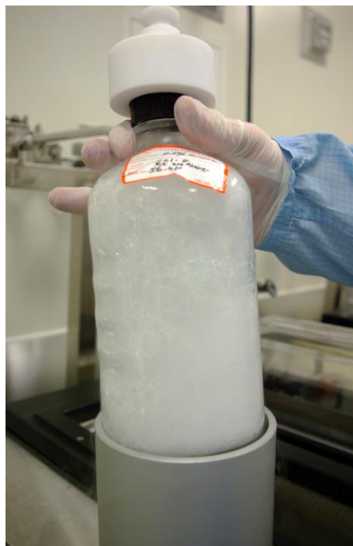
Figure 4-4: Rolleraid cap, 1L bottle placed in aluminum sleeve after shell freezing
