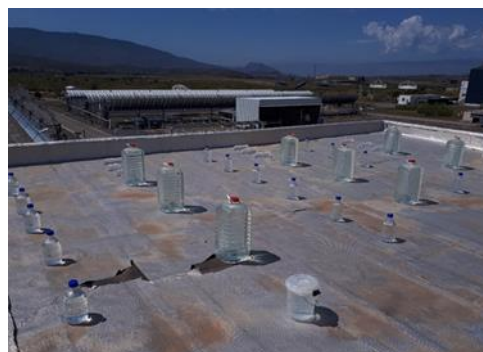
Figure 2.10 PET and PP reactors exposed to the sunlight at PSA
