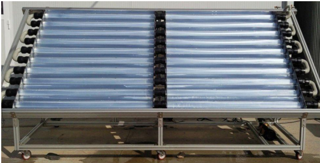
Figure 1.5 SODIS enhanced large batch multitube flow-reactor of 100L with add-on CPC mirrors. Picture taken at Plataforma Solar de Almería, Spain (Polo-López et al., 2011)
