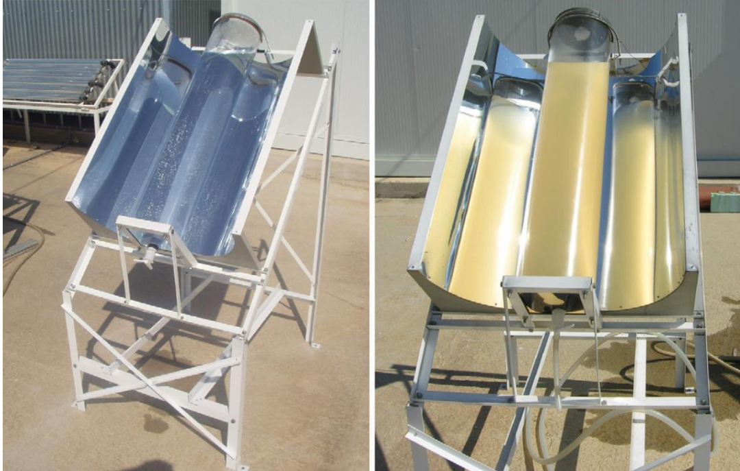
Figure 1.6. SODIS enhanced large batch reactor of 25 L, with a solar mirror. Picture taken at Plataforma Solar de Almería, Spain (Ubomba-Jaswa et al., 2009)
