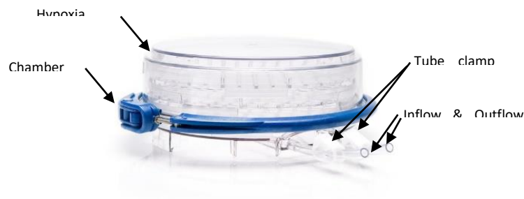
Figure 2.3: Hypoxic chamber with inflow and outflow tube fitted with tube clamp clips and sealing chamber clamp.
