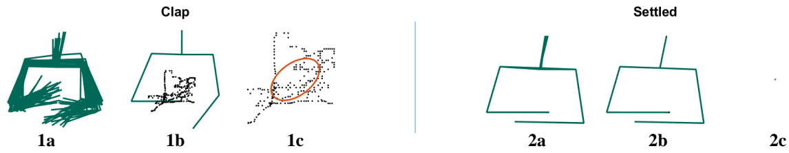
Figure 6. A covariance ellipse can be used to describe movement. Whilst the wrist movement of clapping is seen the large ellipse 1c (plotted in red), no movement, as in 2c, produces a tiny ellipse.
