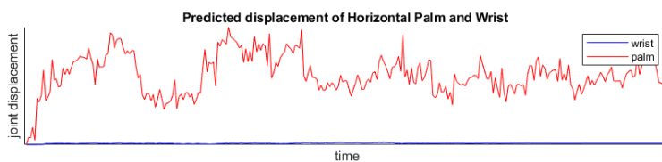
Figure 3: The difference between the extent of palm and wrist movement suggests erroneous keypoint predictions.
