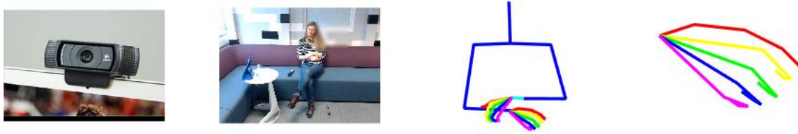
Figure 8: With a camera placed above the TV screen, the subject is recorded whilst seated, watching TV. OpenPose is used to estimate hand and body keypoints.
