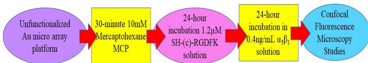
Figure 4.16: Schematic showing experimental set-up using \alpha_5\beta_1 incubation for confocal fluorescence microscopic studies as further confirmation of successful SH-(c)-RGDFK functionalization.
