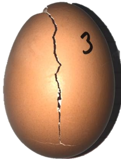
Figure 4.2.2. Fracture in eggshell occurring vertically along from preformed notch.
