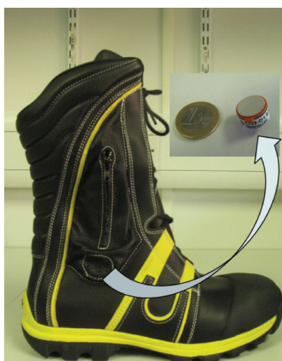
Figure 1: Firefighter's boot with built-in pocket used for enclosing the CO 2 sensor and wireless communications platform.
