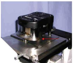
FIGURE 2.2(B): AFM MOUNT ASSEMBLY. THE SAMPLE IS PLACED APPROXIMATELY WHERE THE RED ARROW INDICATES 13.
