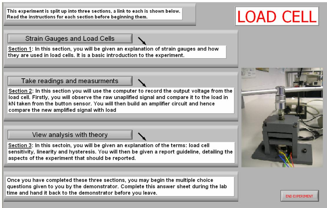
Figure 1: Main menu of Load Cell experiment
