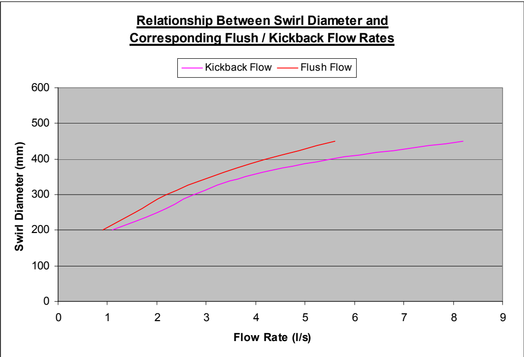
Figure 4.17 – Swirl Diameter and Flush Flow / Kickback Flow Relationship
