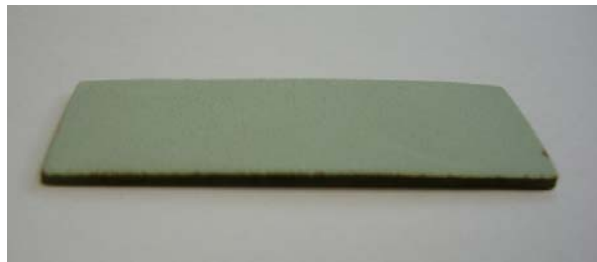
Figure 4.12: Green appearance of coating after heat treatment at 800 °C for 2 hours
