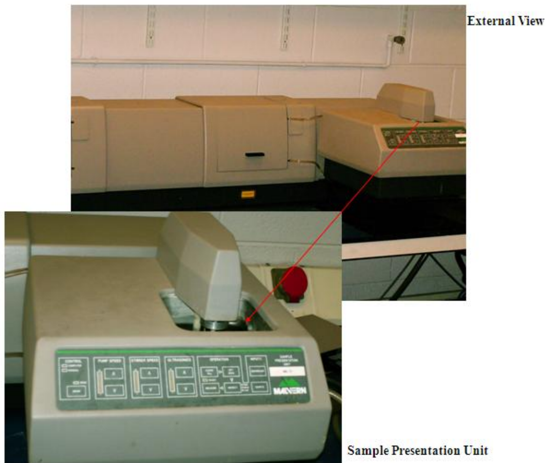
Figure 3-14: External view of the Malvern Mastersizer particle size analyser and sample preparation unit
