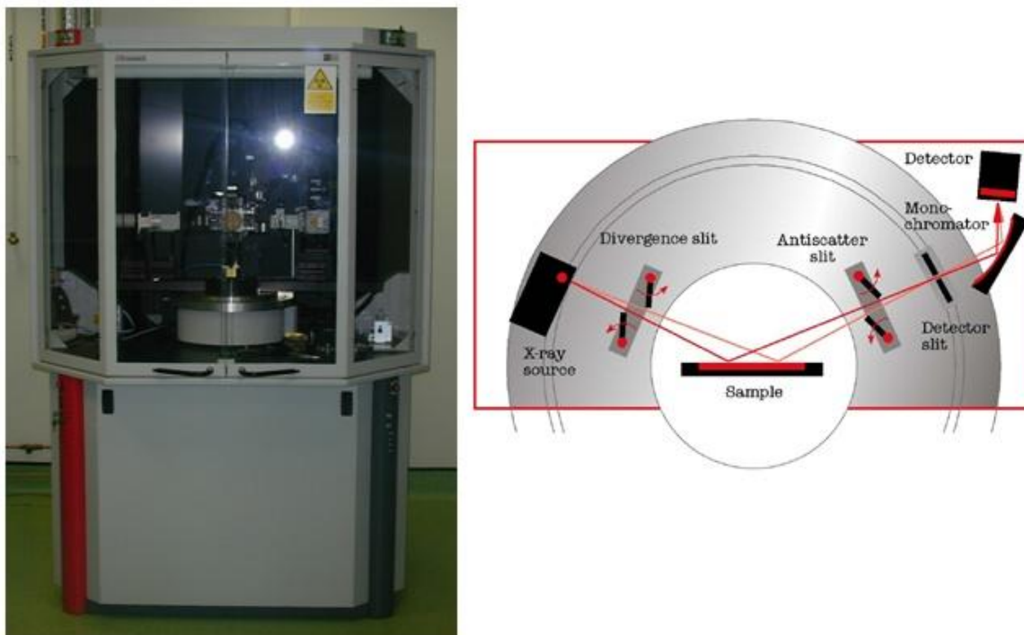
Figure 3-11: Bruker AXS D8 Advance XRD in the Materials Research Processing Centre, MPRC (left hand side) and typical features of the XRD equipment (right hand side)
