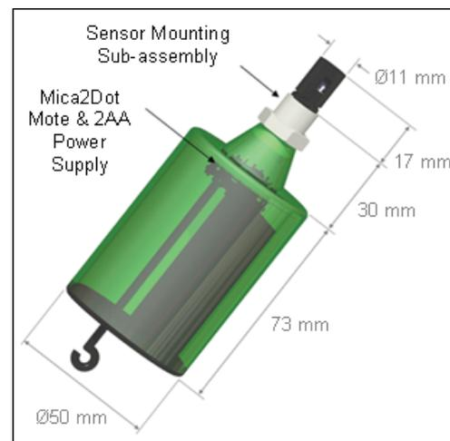
Fig. 1 – The wireless sensor node
