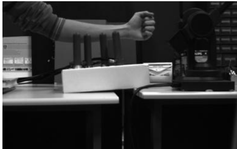
Figure 5.25: Heat emitting body near teat ends
