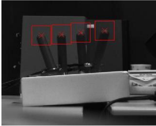
Figure 5.6: Results of homography in right image & ROI for each teat- situation 1
