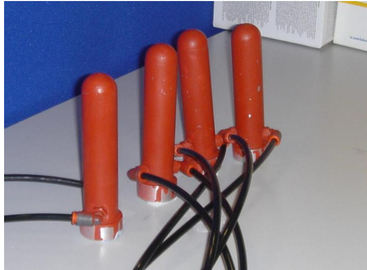
Figure 3.9: Thermal dummy teats
