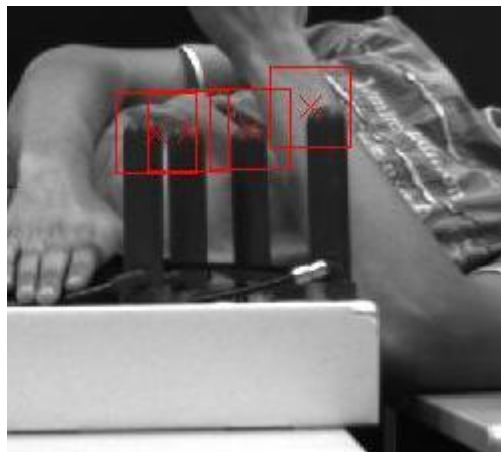
Figure 5.29: Results of homography in left image & ROI for each teat- Situation 6
