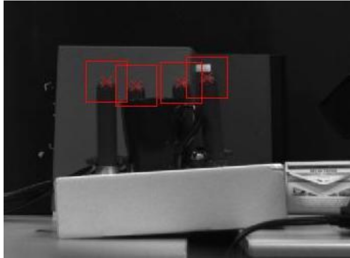
Figure 5.22: Results of homography in right image & ROI for each teat- situation 4
