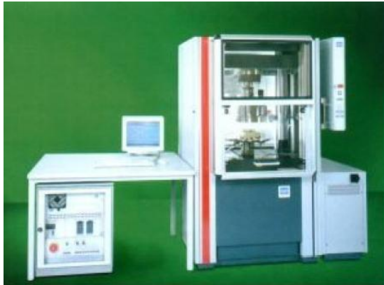
Figure 3.2: Hot Embossing model HEX 02 from Jenoptik
