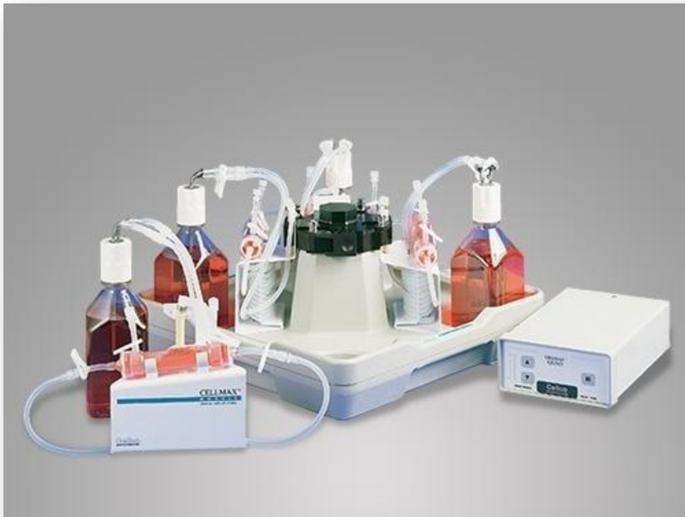
Figure 2.12 CellMax Hollow Fibre Bioreactor for co-culture of Smooth Muscle cells and endothelial cells on hollow fibres, which provide the physical segregation of the cell types. Pulsatile flow is obtained by a pump system and 4 bioreactors can be run simultaneously (Image is obtained from Spectrum Labs Inc. website, www.spectrumlabs.com ).
