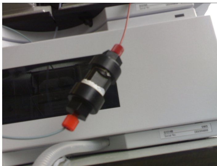
Figure 4.12. Typical 5 \mu m macro-porous carbon monolithic column (30 x 6 mm i.d.).
