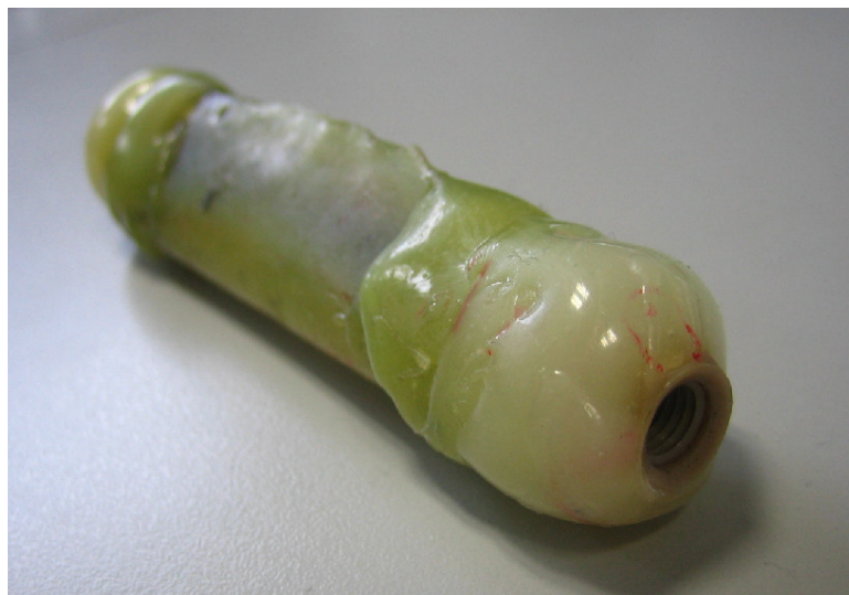
Figure 4.21. The typical image of the 1 \mu\text{m} templated carbon monolithic column (73 x 4 mm i.d.) encased within epoxy resin.
