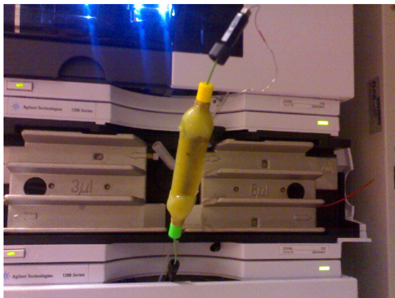
Figure 4.17. The typical image of the carbon monolithic column (1 \mu\text{m} pore diameter), 75 x 6 mm i.d encased within epoxy resin.
