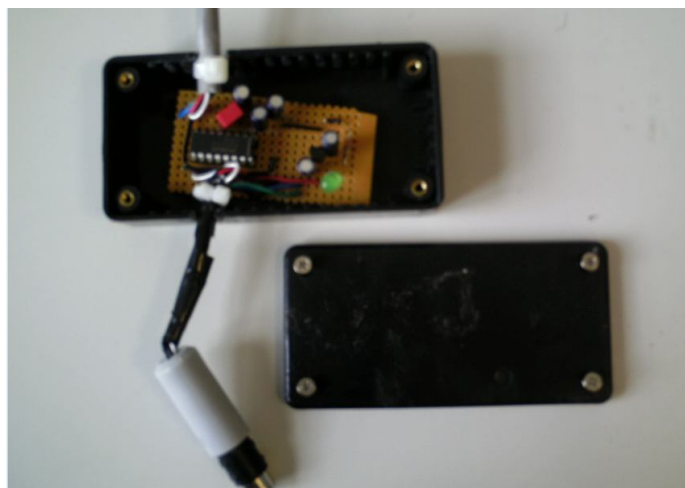
Figure 8: Photo of Power Regulator/Serial Cable
