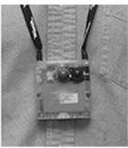
Figure 1. The Microsoft Sensecam, inset as worn by a user. (Adapted from Microsoft Research SenseCam homepage).
