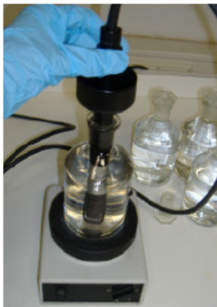
Fig. 1.3: Dissolved oxygen analysis carried out on the closed bottles. 34
