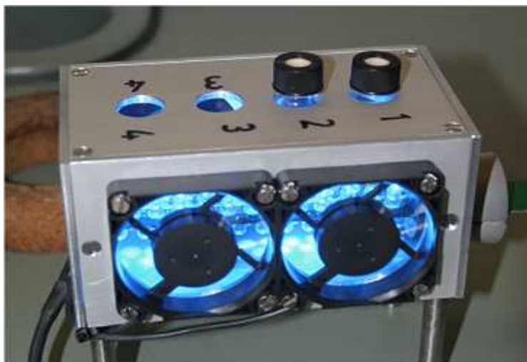
Figure 2.18 shows the reactor where the catalytic solutions were irradiated by blue LEDs (470 nm wavelength).
