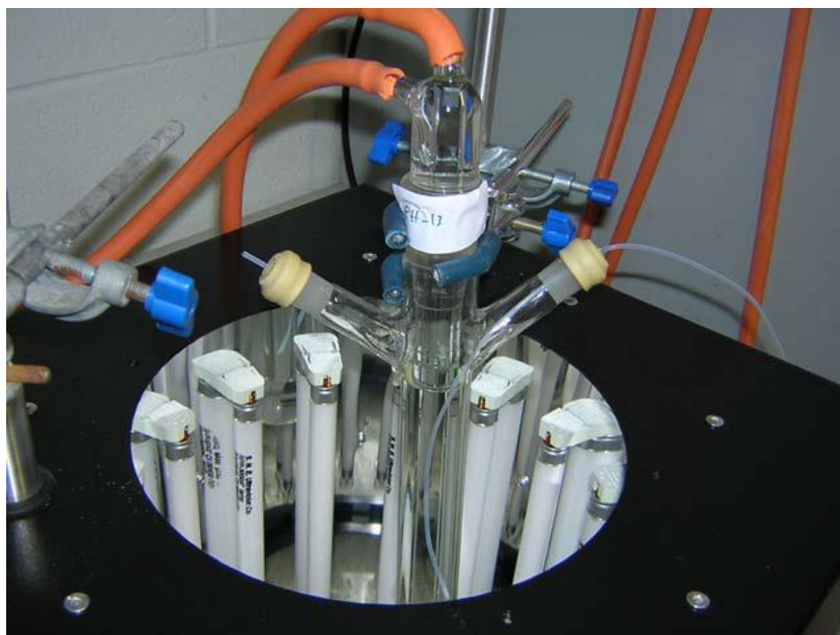
Figure 4.3 Rayonet photochemical reactor (RPR-200) equipped with 16 RPR 3000Å lamps, used in the synthesis of 2,4,5,8,-tetraphenyl-2,5,6,7-tetrahydro-1,2,3,5-tetrazocines ( 43 ) and of imidazo-[4,5- c ]pyrazoles( 47 ).
