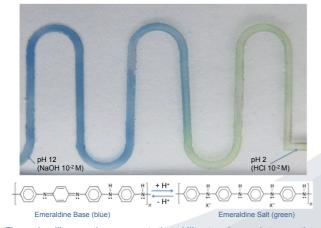
The polyaniline coatings present the ability to change between the emeraldine salt form of PAni (green) to the emeraldine base form (blue) when a solution of HCI 10<sup>-2</sup> M, NaOH 10<sup>-2</sup> M respectively, is flushed inside the channel. Moreover, the PAni coatings shows dynamic response throughout the entire length of the channel.
