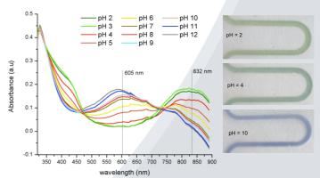
The optical/electrical proprieties of these polyaniline coatings change in response to the pH of the solution that is flushed inside the micro-channel.
