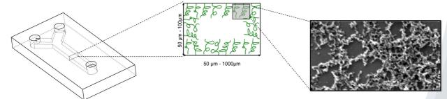
Polymer brushes based on the conducting polymer polyaniline were synthesised on the interior walls of micro-fluidic devices.
