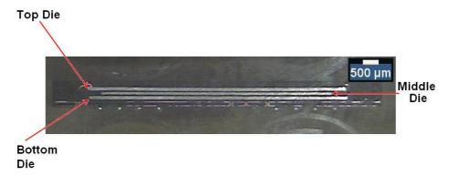
Figure 6.3(a): Optical cross section of stacked CSP enclosed in resin, showing 3-layer structure. Total package height ~675  $\mu$ m (excluding BGA), die thickness ~100  $\mu$ m. Die stack thickness ~350  $\mu$ m. Bottom die is attached to substrate by adhesive.
