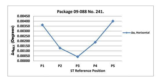
Figure 5.33: Angular displacement (warpage) data for package 09-088 No. 241. Horizontal ST topograph positions (P1 – P5) correspond to red lines in Figure 3.14.
