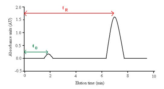
Figure 1.1: Schematic of a typical HPLC chromatogram
