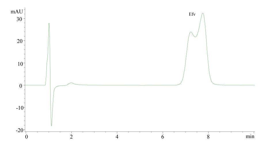
Figure 2.3: Chromatogram of a working standard of Efv using an Agilent Zorbax SB-C18 column
