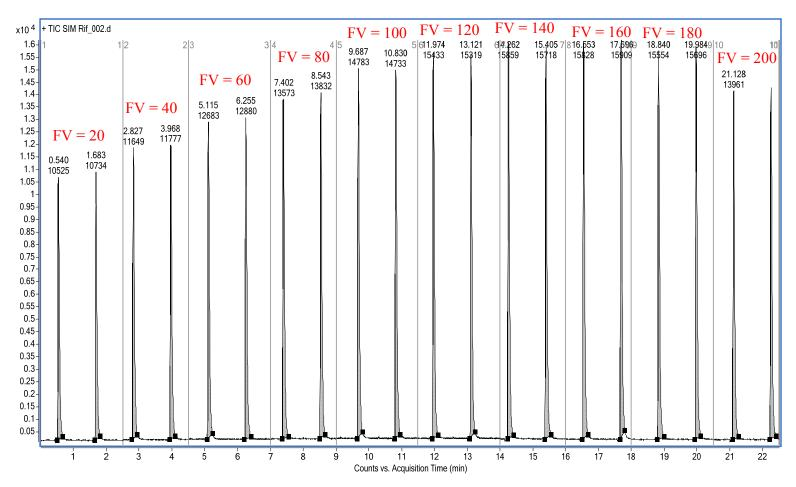
Figure 3.4: TIC for *m/z* of 823.4 for Rif in SIM mode with increasing fragmentor voltage
