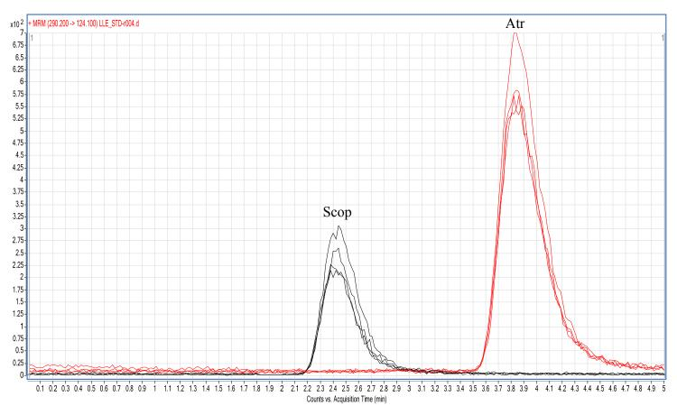
Figure 4.33: LC-MS chromatogram, in MRM mode, of Scop and Atr std in MP brought through the LLE extraction process (no serum) using an Agilent Zorbax SB-C18 column
