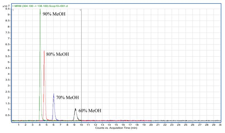
Figure 4.43: Comparison of the impact of different different % MeOH mobile phase compositions on peak shape and retention for Scop using an Agilent Zorbax SB-Phenyl column
