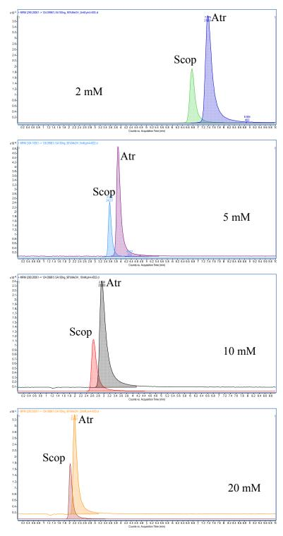
Figure 4.14: Comparison of the impact of different ammonium formate concentrations (pH 5) on peak shape and retention for Scop and Atr using a Waters Nova-Pak C18 column
