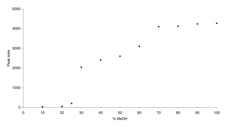
Figure 4.46: Comparison of different MeOH compositions in the SPE wash step on the retention of Scop
