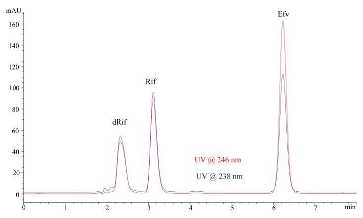
Figure 2.8: Chromatogram of a working standard of Efv and Rif prepared to  $10~\mu\text{g/mL}$  in mobile phase under the final chromatographic conditions
