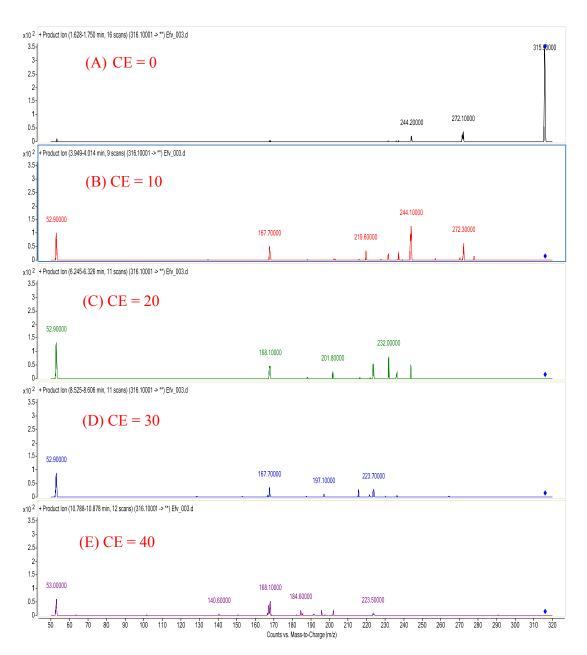
Figure 3.7: TIC for the product ion scan of Efv with increasing collision energies
