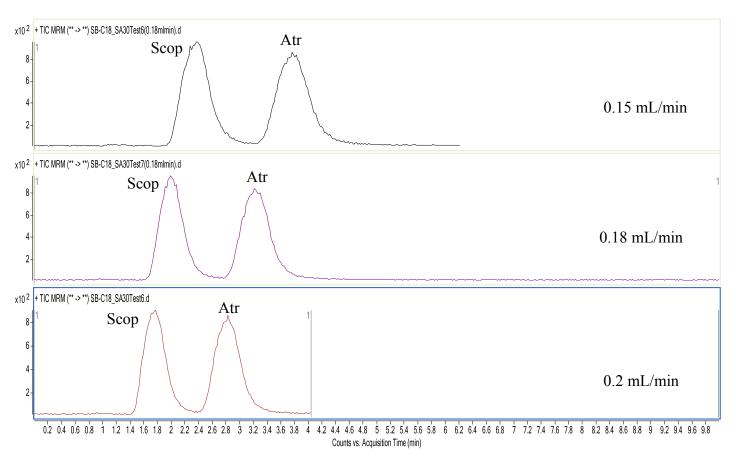
Figure 4.21: Comparison of the impact of different flowrates on peak shape and retention for Scop and Atr using an Agilent Zorbax SB-C18 column
