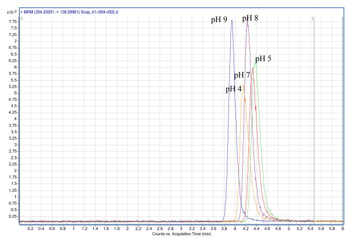
Figure 4.45: Comparison of the impact of different mobile phase pHs using 10 mM ammonium formate on peak shape and retention for Scop using an Agilent Zorbax SB-Phenyl column
