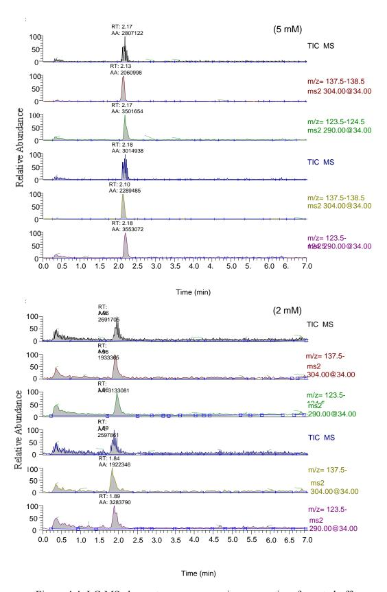
Figure 4.4: LC-MS chromatograms comparing ammonium formate buffer concentrations for a 10 ng/mL Scop and Atr standard using an Agilent Zorbax SB-CN column
