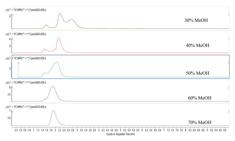
Figure 4.10: Comparison of the impact of different % MeOH mobile phase compositions on peak shape and retention for Scop and Atr using an Agilent Zorbax SB-CN column
