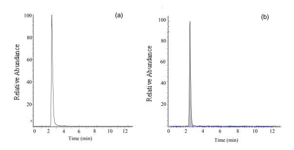
Figure 4.9: MRM chromatograms of a) extracted serum sample spiked with 10 ng/mL Scop and b) a working standard of Scop prepared to 10 ng/mL in mobile phase using an Agilent Zorbax SB-CN column
