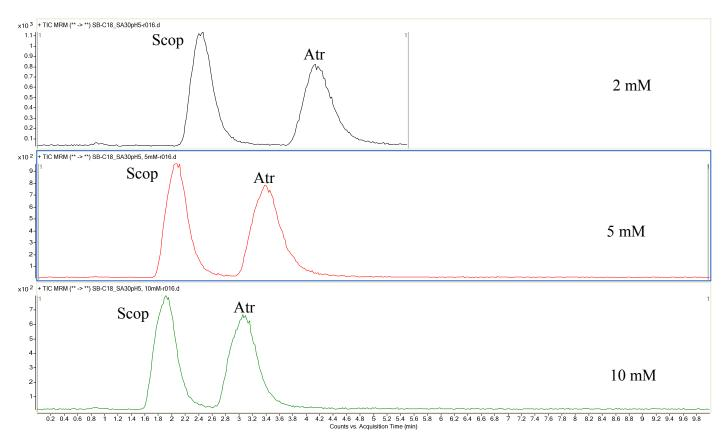
Figure 4.23: Comparison of the impact of different ammonium formate concentrations (pH 4) on peak shape and retention for Scop and Atr using an Agilent Zorbax SB-C18 column
