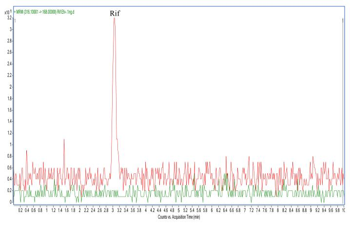
Figure 3.15: Chromatogram of a working standard of Rif prepared to 1 ng/mL in plasma
