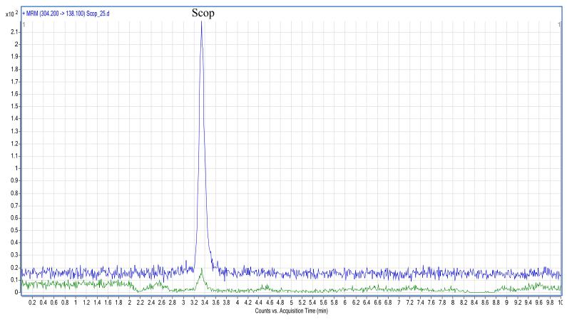
Figure 4.26: Serum blank extracted and reconstituted in 1 ng/mL standard of Scop (green) superimposed on the pure 1 ng/mL standard (blue) using an Agilent Zorbax SB-C18 column
