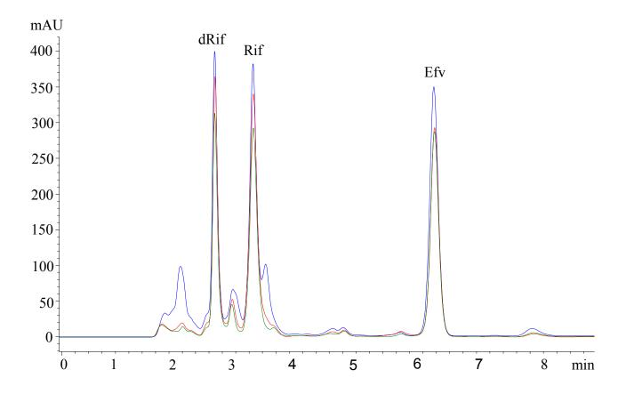
Figure 2.12: Chromatogram comparing different plasma load conditions for Efv.
