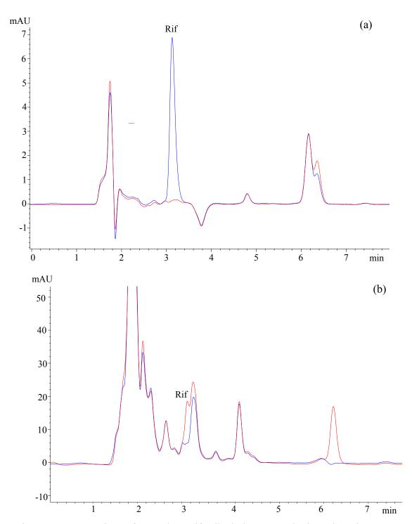
Figure 2.9: Comparison of a 1  $\mu$ g/mL Rif spiked plasma standard monitored at (a) 334 nm and (b) 238 nm
