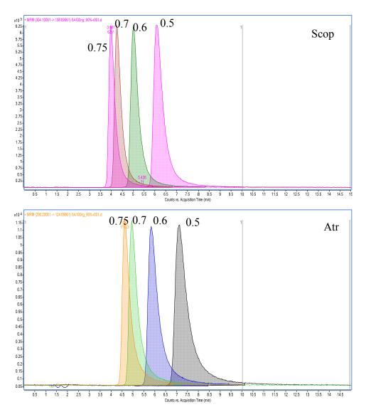
Figure 4.17: Comparison of the impact of different flowrates on peak shape and retention for Scop and Atr using a Waters Nova-Pak C18 column
