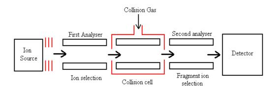
Figure 1.6: Schematic of the Triple Quadrupole Mass Spectrometer
