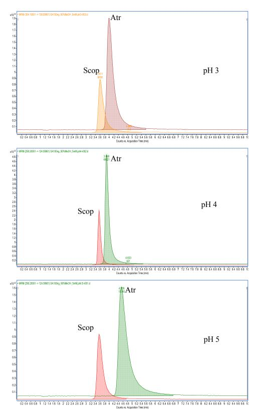
Figure 4.16: Comparison of the impact of different mobile phase pHs using 5 mM ammonium formate on peak shape and retention for Scop and Atr using a Waters Nova-Pak C18 column
