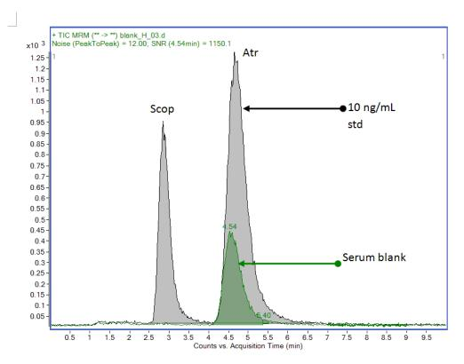
Figure 4.25: Overlay of a 10 ng/mL Scop and Atr standard in MP (grey) superimposed on extracted serum blank (green) using an Agilent Zorbax SB-C18 column
