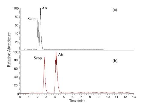
Figure 4.3 Chromatograms comparing the separation of Scop and Atr using (a) a Supelcosil LC-18 column and (b) an Agilent Zorbax SB-CN column
