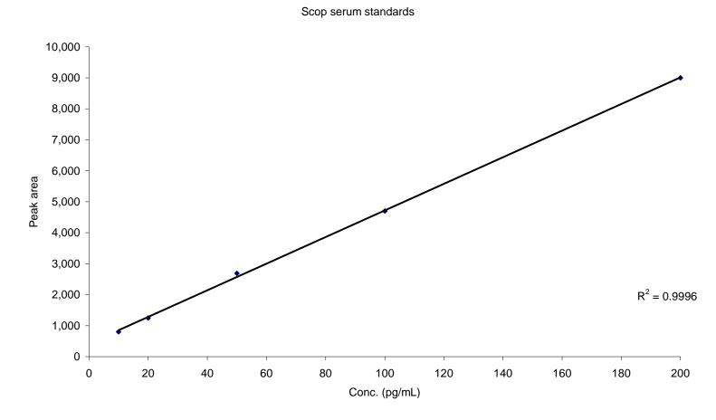
Figure 4.52: Linearity for Scop serum standards using an Agilent Zorbax SB-Phenyl column
