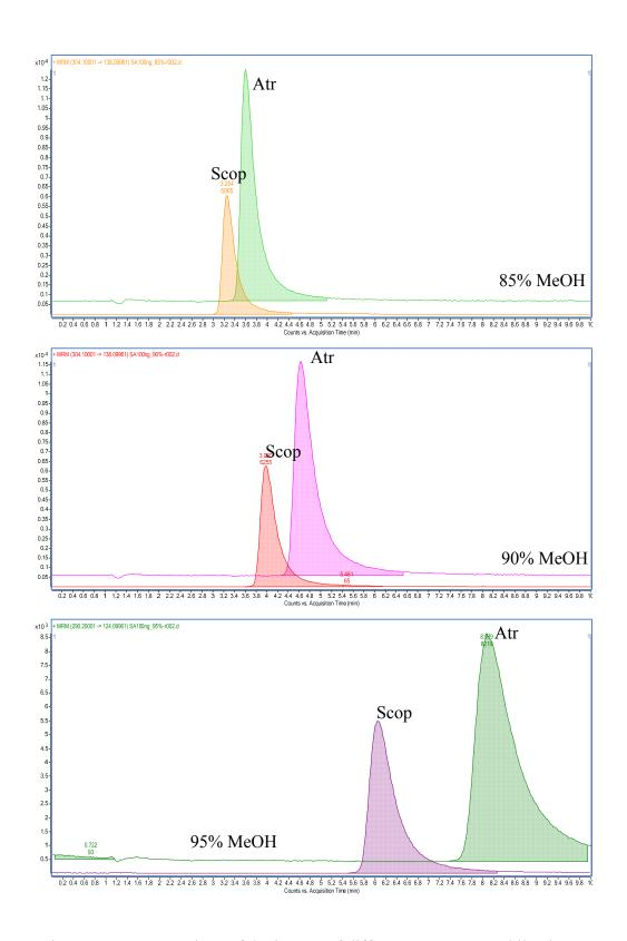
Figure 4.13: Comparison of the impact of different % MeOH mobile phase compositions on peak shape and retention for Scop and Atr using a Waters
