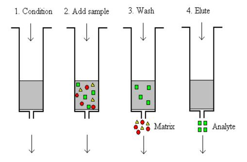
Figure 1.7: Schematic showing the four main steps in a typical SPE procedure
