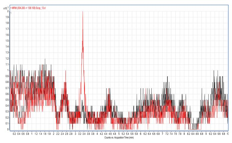
Figure 4.28: Chromatogram of an extracted serum blank superimposed on an extracted 100 pg/mL serum standard extracted using an Agilent Zorbax SB-C18 column
