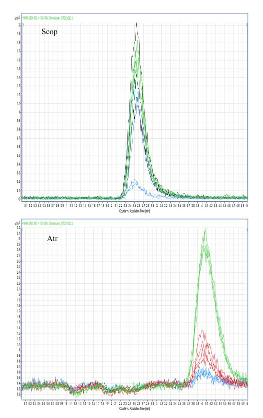
Figure 4.29: LC-MS chromatogram, in MRM mode of an extracted serum blank sample (blue) and an extracted spiked serum Scop standard (black) and Atr (red) superimposed on a pure std of both drugs in MP (green) using chlorobutane as extraction solvent
