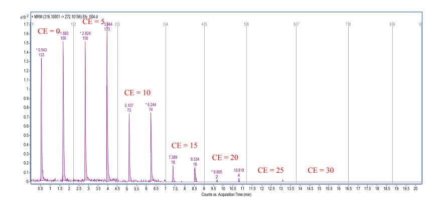
Figure 3.13: Efv product ion m/z 272.1 with increasing collision energies
