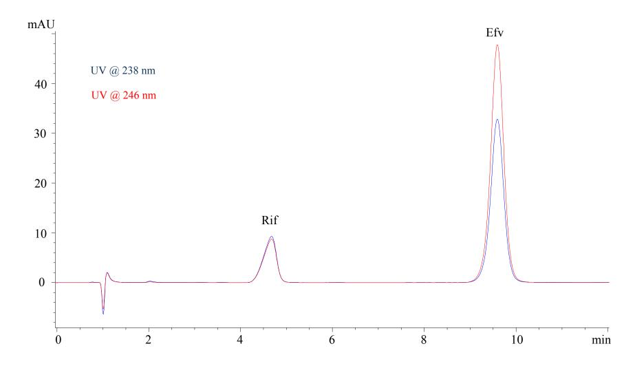
Figure 2.4: Chromatogram of a working standard of Rif and Efv using a Varian pursuit column
