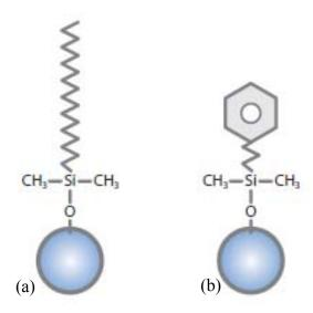
Figure 2.2: Reversed phase stationary phases (a) C18 and (b) phenyl
