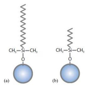
Figure 4.38: Reversed phase stationary phases (a) C18 and (b) C8
