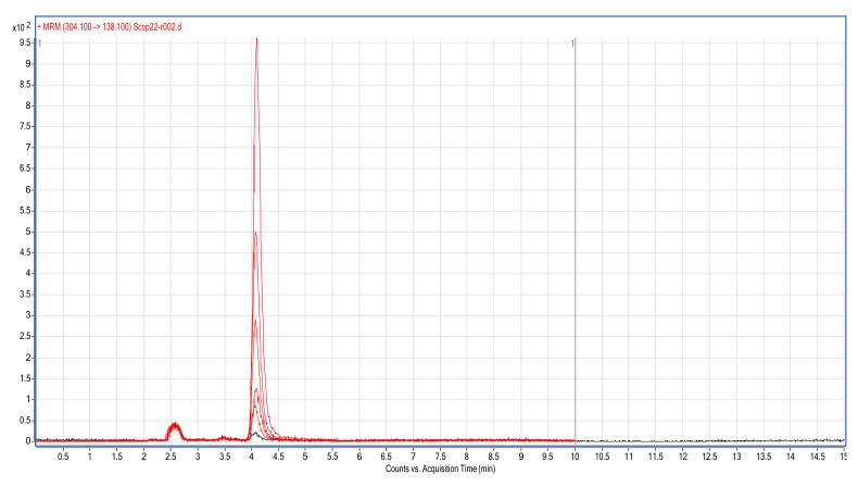
Figure 4.51: Chromatograms of extracted drug-free serum sample (black) superimposed on extracted serum spiked with 10, 20, 50, 100 and 200 pg/mL Scop (red) using an Agilent Zorbax SB-Phenyl column
