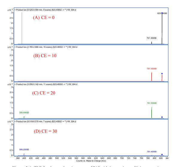
Figure 3.6: TIC for the product ion scan of Rif with increasing collision energies
