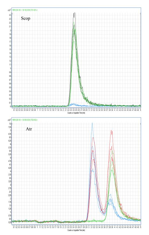
Figure 4.30: LC-MS chromatogram, in MRM mode of an extracted serum blank sample (blue) and an extracted spiked serum Scop standard (black) and Atr (red) superimposed on a pure std of both drugs in MP (green) using DCM as extraction solvent
