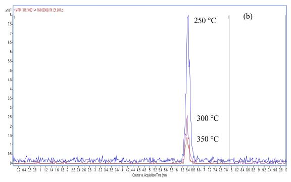
Figure 3.14: Comparison of different capillary temperatures for (a) Rif and (b) Efv
