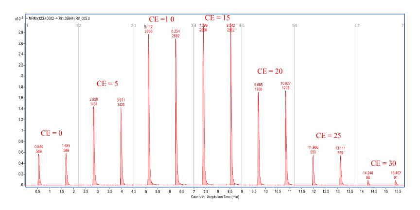
Figure 3.8: Rif product ion m/z 791.3 with increasing collision energies
