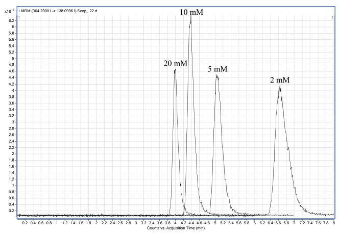
Figure 4.44: Comparison of the impact of different ammonium formate concentrations (pH 5) on peak shape and retention for Scop using an Agilent Zorbax SB-Phenyl column
