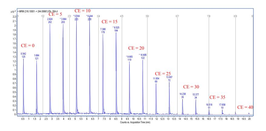
Figure 3.12: Efv product ion m/z 244.1 with increasing collision energies
