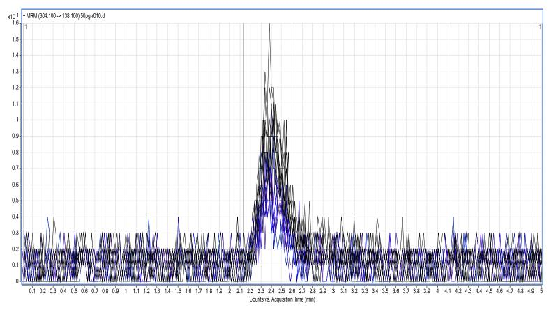
Figure 4.37: LC-MS chromatogram, in MRM mode of extracted spiked (200 pg/mL) serum standard (black) superimposed on extracted serum blank sample (blue) using an Agilent Zorbax SB-C18 column
