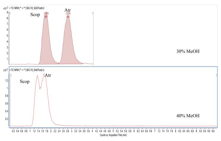
Figure 4.22: Comparison of the impact of different % MeOH mobile phase compositions on peak shape and retention for Scop and Atr using an Agilent Zorbax SB-C18 column
