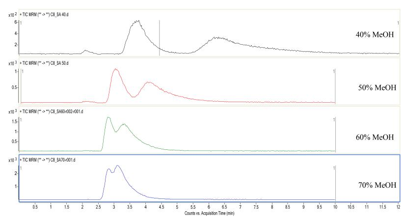
Figure 4.39: Comparison of the impact of different % MeOH mobile phase compositions on peak shape and retention for Scop and Atr using an Agilent Zorbax RX-C8 column
