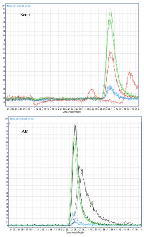
Figure 4.32: LC-MS chromatogram, in MRM mode of an extracted serum blank sample (blue) and an extracted spiked serum Scop standard (red) and Atr (black) superimposed on a pure std of both drugs in MP (green) using *tert*-butyl methyl ether as extraction solvent
