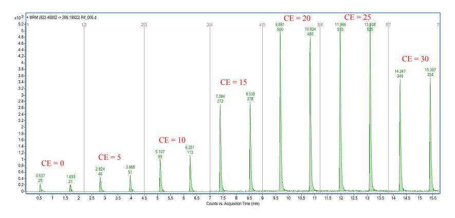
Figure 3.9: Rif product ion m/z 399.2 with increasing collision energies
