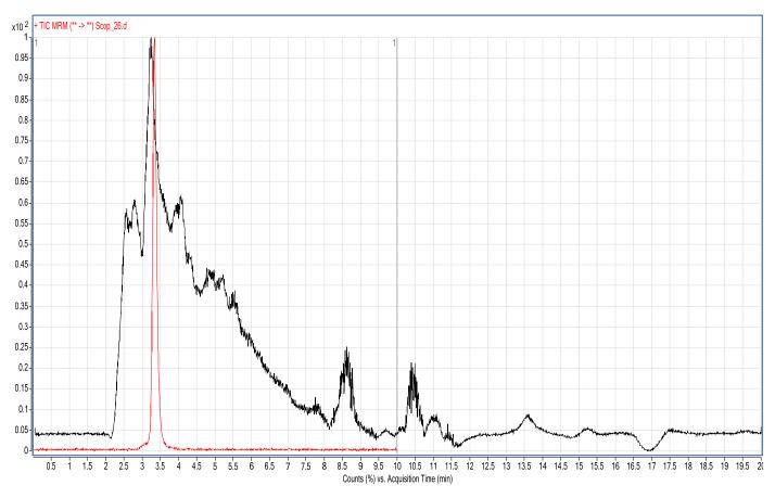
Figure 4.27: TIC scan of serum blank extracted (black) superimposed on a MRM scan of Scop pure standard (red) using an Agilent Zorbax SB-C18 column. Note: not to scale
