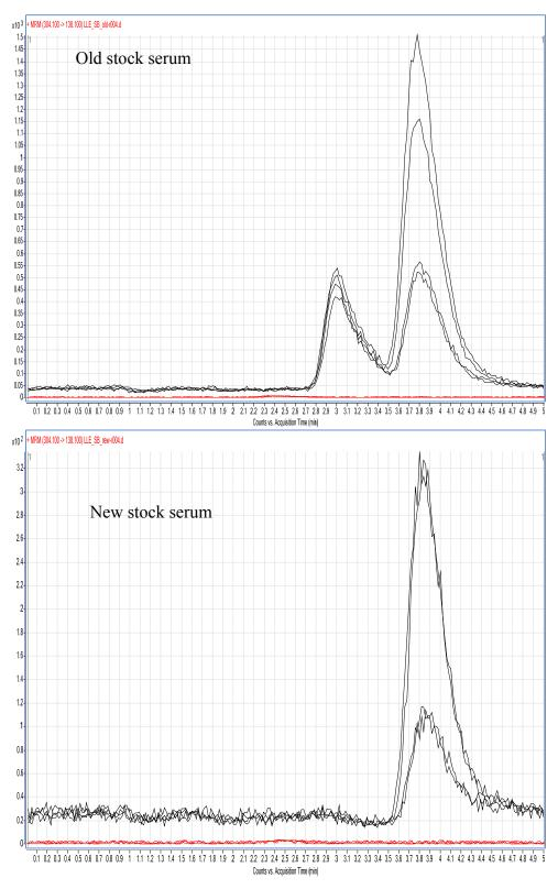
Figure 4.34: LC-MS chromatograms, in MRM mode comparing LLE extracted blank serum for old and new serum batches using an Agilent Zorbax SB-C18 column
