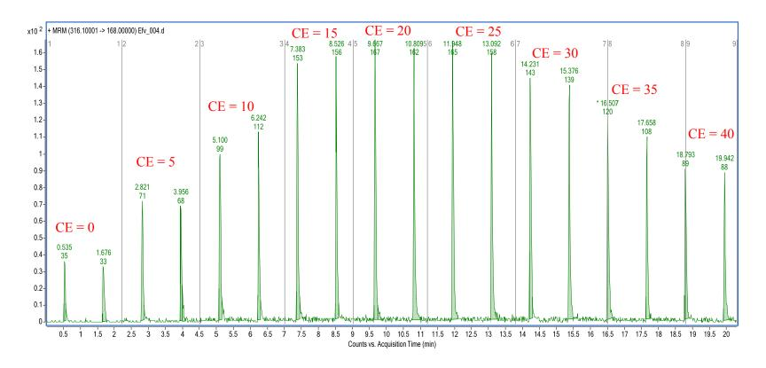
Figure 3.11: Efv product ion m/z 168.0 with increasing collision energies
