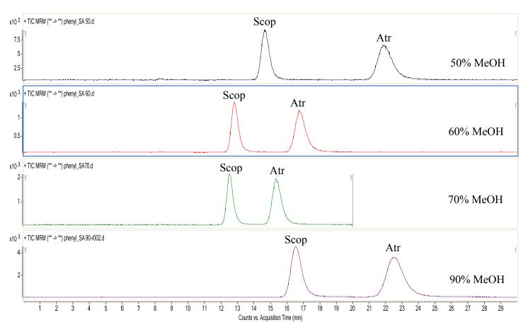
Figure 4.42: Comparison of the impact of different % MeOH mobile phase compositions on peak shape and retention for Scop and Atr using an Agilent Zorbax SB-Phenyl column
