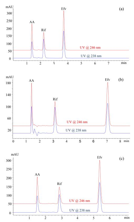
Figure 2.6: Chromatograms of a 10  $\mu$ g/mL standard of ascorbic acid (AA), Efv and Rif prepared in mobile phase using various mobile phase compositions of H<sub>2</sub>O-ACN-MeOH (a) 35:50:20, v/v/v (b) 45:40:15, v/v/v and c) 40:45:15, v/v/v.
