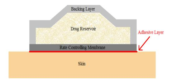
Figure 5.1: Diagrammatic representation of the cross section of the transdermal Scop patch
