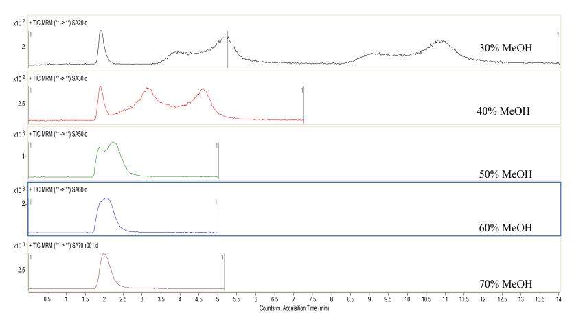
Figure 4.11: Comparison of the impact of different % MeOH mobile phase compositions on peak shape and retention for Scop and Atr using an Agilent Zorbax RX-C18 column
