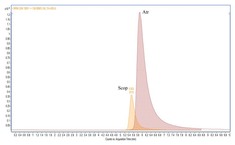
Figure 4.15: Chromatogram of Scop and Atr using 0.1% formic acid as mobile phase using a Waters Nova-Pak C18 column
