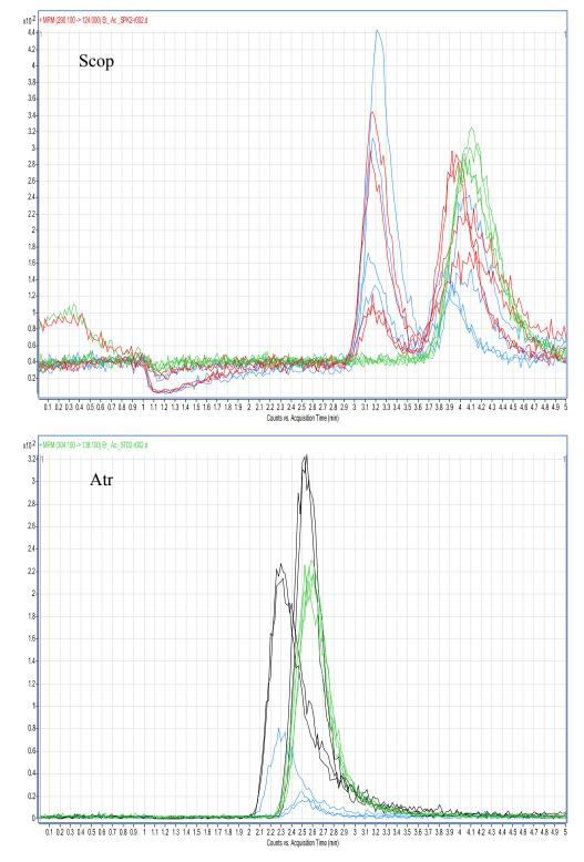
Figure 4.31: LC-MS chromatogram, in MRM mode of an extracted serum blank sample (blue) and an extracted spiked serum Scop standard (red) and Atr (black) superimposed on a pure std of both drugs in MP (green) using ethyl acetate as extraction solvent
