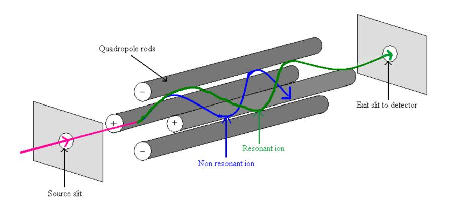
Figure 1.5: Adapted schematic of a Quadrupole Mass Analyser (Gates, 2009)
