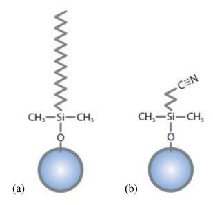
Figure 4.2: Reversed phase stationary phases (a) C18 and (b) CN
