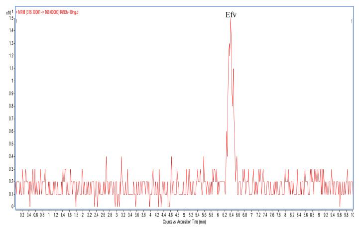
Figure 3.16: Chromatogram of a working standard of Efv prepared to 10 ng/mL in plasma
