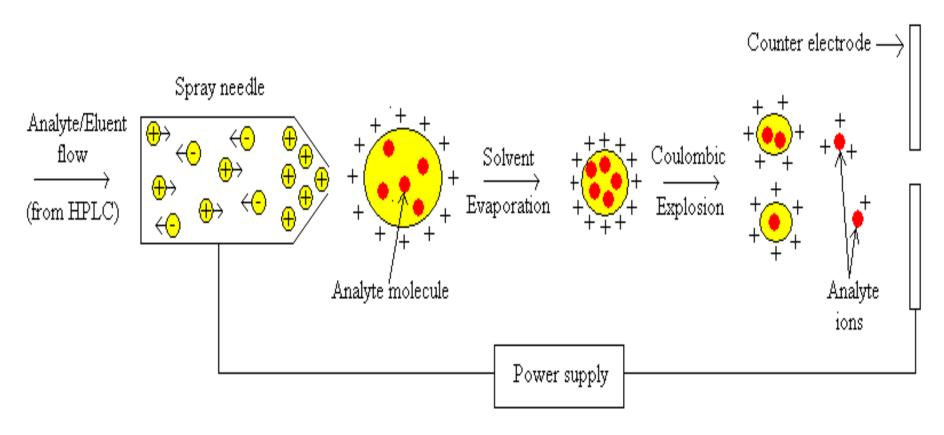
Figure 1.4: Adapted schematic of electrospray ionisation (Gates, 2004)
