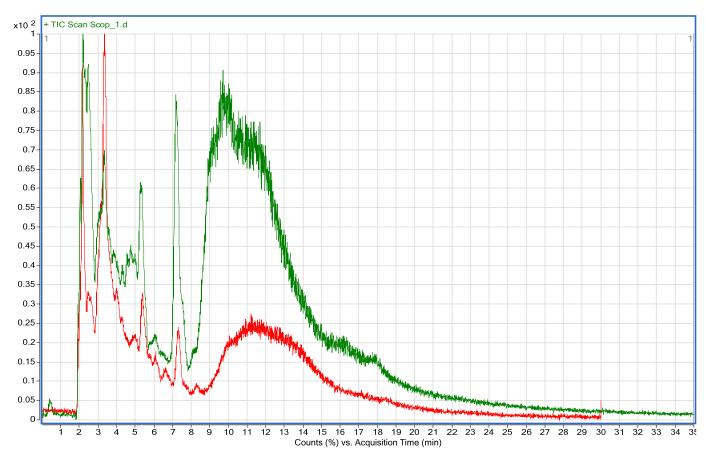
Figure 4.47: TIC scan showing differences between eluting with 100% MeOH (green) and 75% MeOH (red) using an Agilent Zorbax SB-Phenyl column
