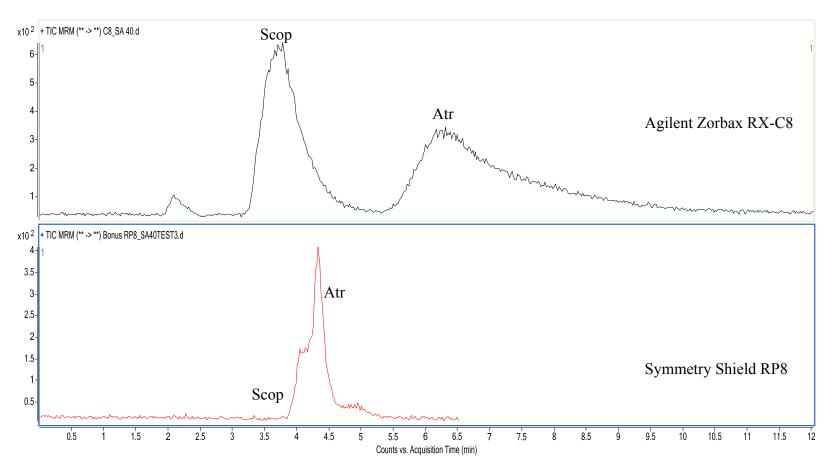
Figure 4.40: Comparison of Agilent Zorbax RX-C8 column to Symmetry Shield RP8 at 40% MeOH
