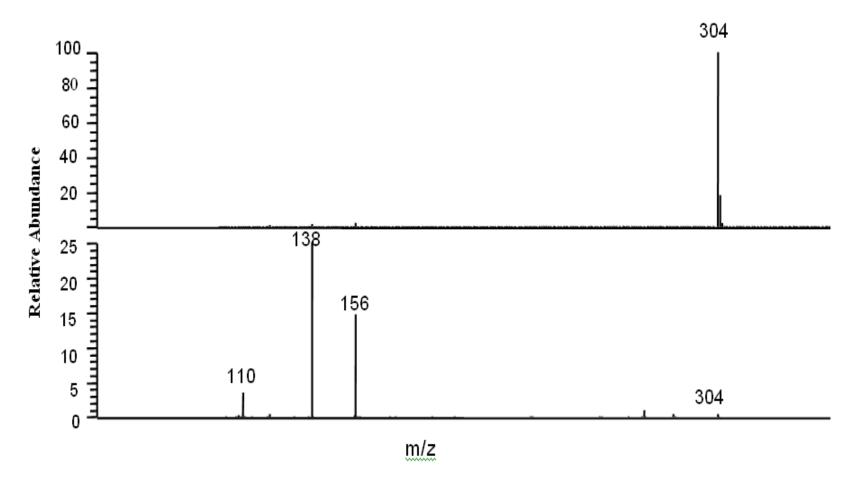
Figure 4.7: The precursor ion and fragment ions of Scop
