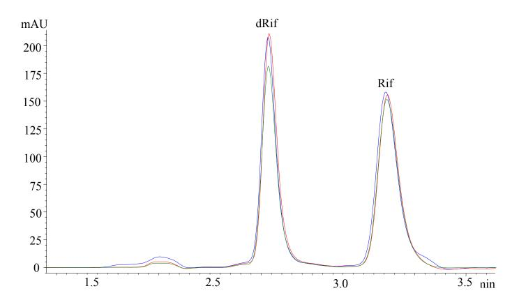
Figure 2.11: Chromatogram comparing different plasma load conditions for dRif and Rif. Blue: 0.1% FA, Red: 0.01% FA Green: water
