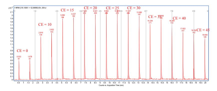
Figure 3.10: Efv product ion m/z 52.9 with increasing collision energies
