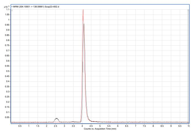
Figure 4.53: Chromatogram displaying ion suppression results. Red: 1ng/ml Scop in MeOH, Black: serum blank reconstituted in the same 1ng/ml Scop standard in MeOH
