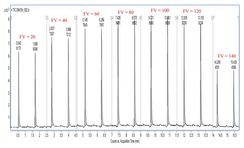
Figure 3.5: TIC for m/z of 316.1 for Efv in SIM mode with increasing fragmentor voltage
