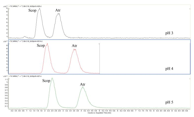
Figure 4.24: Comparison of the impact of different mobile phase pHs using 2 mM ammonium formate on peak shape and retention for Scop and Atr using an Agilent Zorbax SB-C18 column
