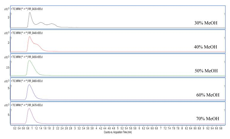
Figure 4.12: Comparison of the impact of different % MeOH mobile phase compositions on peak shape and retention for Scop and Atr using an Agilent Zorbax Eclipse Rapid Resolution column
