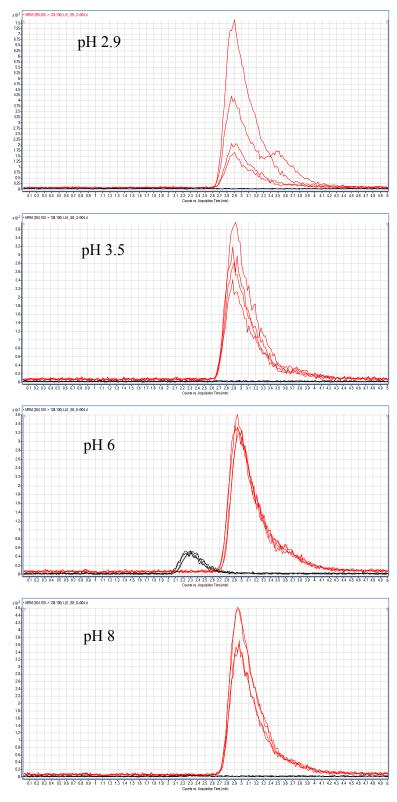
Figure 4.35: LC-MS chromatograms, in MRM mode, comparing the extraction of serum blanks at different pHs using an Agilent Zorbax SB-C18 column (Scop: black, Atr: Red)
