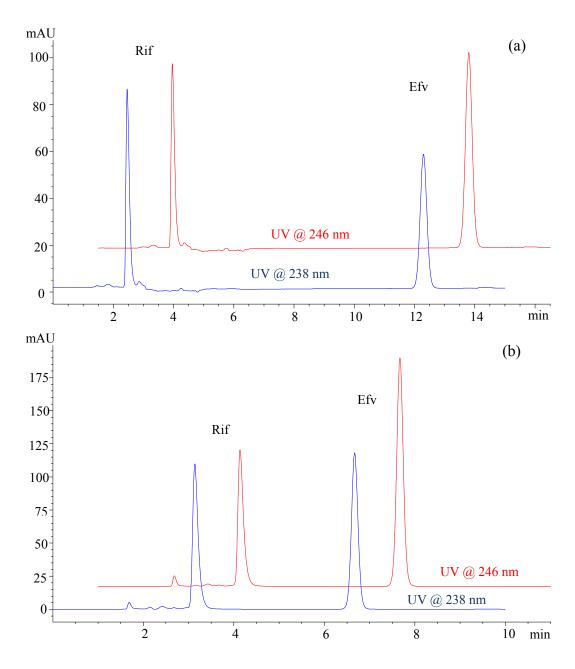
Figure 2.5: Chromatogram of a working standard of Efv and Rif prepared to 10  $\mu$ g/mL in mobile phase comparing (a) the Varian Polaris C18 column and (b) the Agilent Zorbax SB Phenyl column
