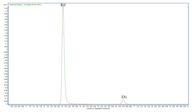
Figure 3.1: Chromatogram of a working standard of Efv and Rif prepared to 500 ng/mL in mobile phase
