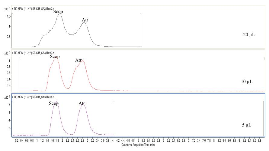
Figure 4.20: Comparison of the impact of different injection volumes on peak shape for Scop and Atr using an Agilent Zorbax SB-C18 column
