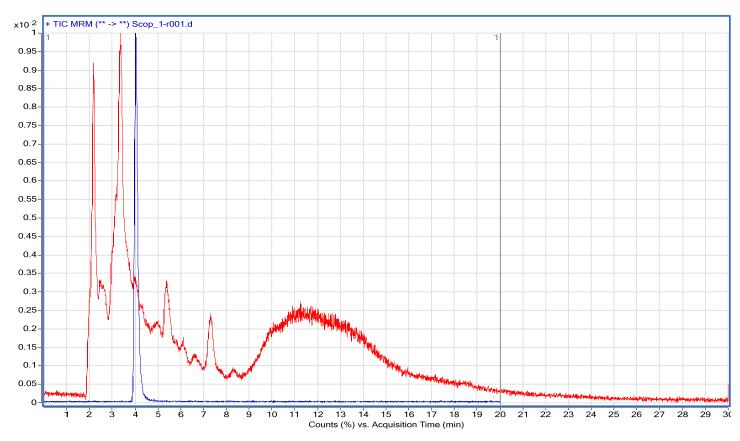
Figure 4.48: Chromatogram of TIC scan of spiked serum sample (red) superimposed on MRM scan of same Scop sample (blue) using an Agilent Zorbax SB-Phenyl column. Note: not to scale
