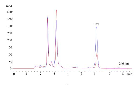
Figure 2.13: Comparison of elution with (blue)  $H_2O$ -ACN-MeOH, 25:50:25 v/v/v, and (red) mobile phase ( $H_2O$ -ACN-MeOH, 40:45:15, v/v/v)
