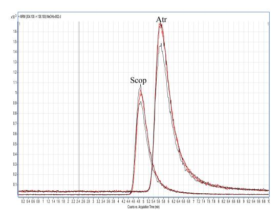
Figure 4.18: Chromatogram of Scop and Atr standard prepared in MP (10 ng/mL) using a Waters Nova-Pak C18 column
