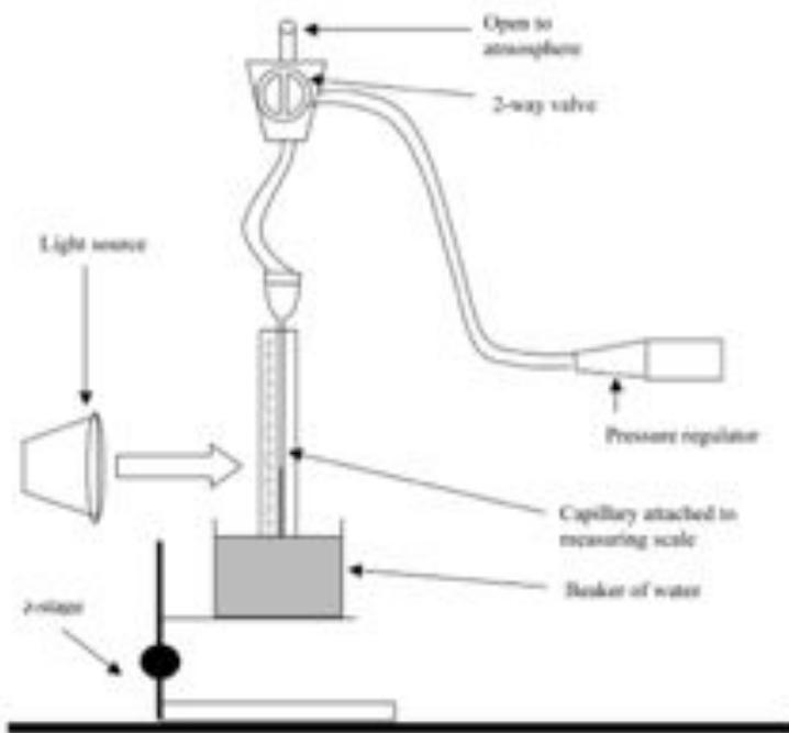
Experimental setup for measurement of capillary rise in a spiropyran monolayer functionalised capillary [1].
