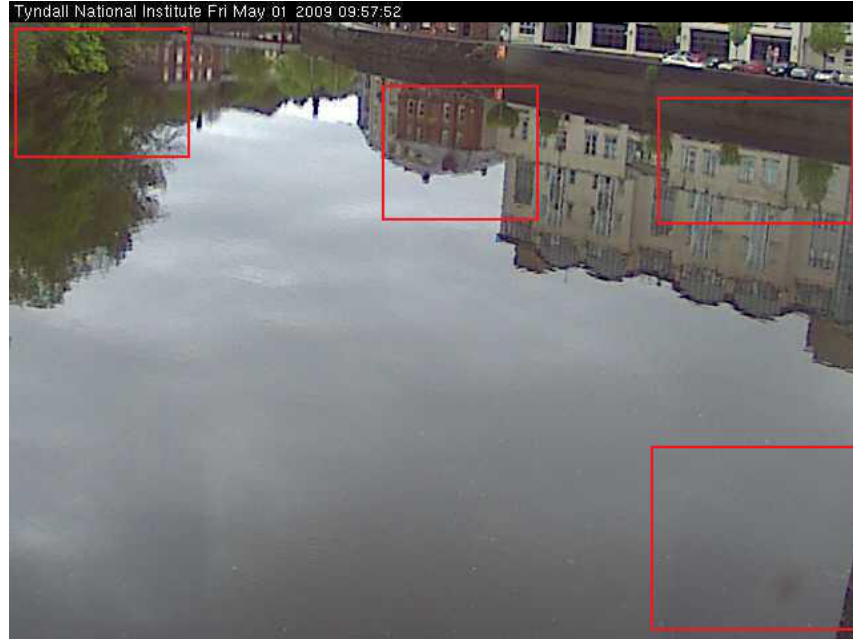
Figure 4.6: Image where none of the depth features are present. It also demonstrates huge image processing challenges with reflections on water and changes in lighting.
