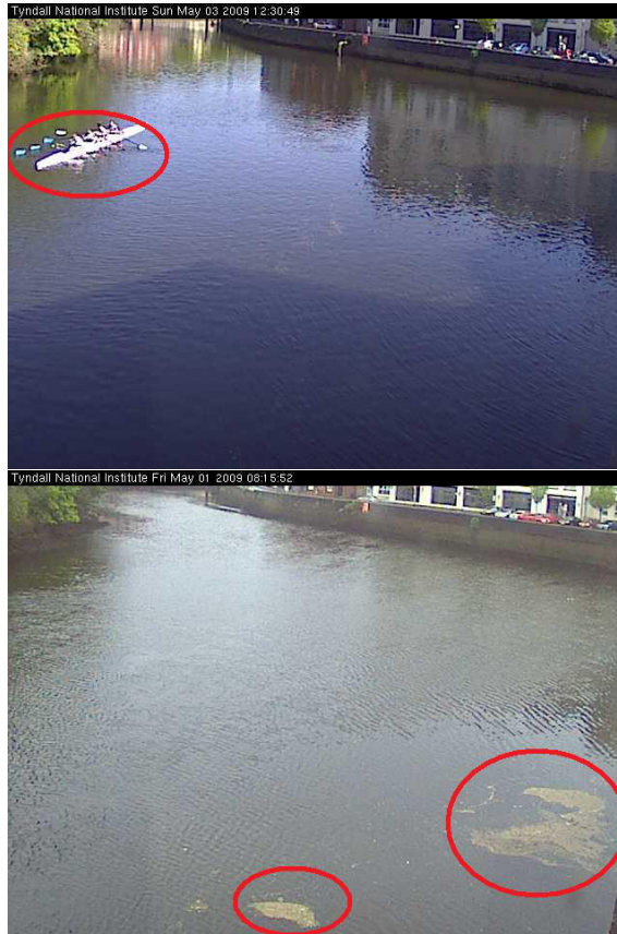
Figure 4.2: A boat on the river and scum floating on the top of the water. Our visual sensing system can detect objects such as these floating on the top of the water
