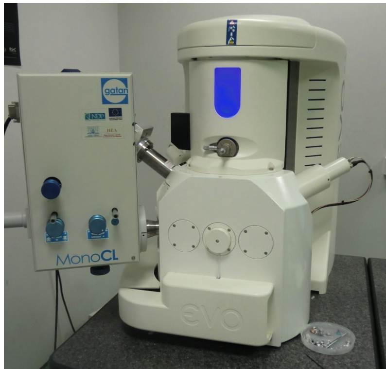
Figure 2.22 CCD image of the SEM system used for measurement. The attached CL and EDX equipment can be seen on the left side of the picture
