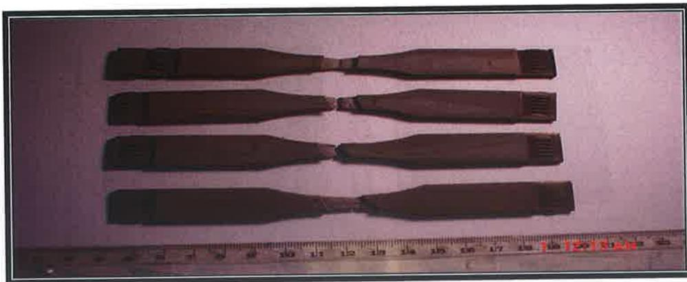
Figure B39: Stainless steel specimens after one (1) week exposure to brine solution tensile tested.
