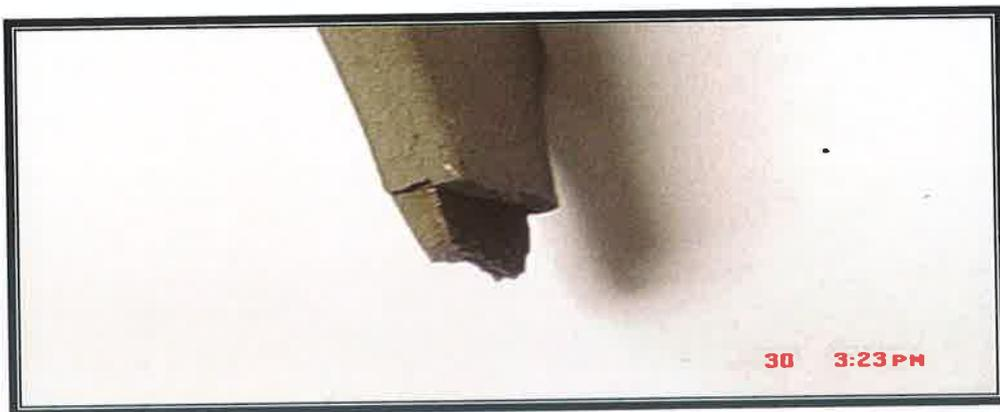
Figure B18: Carbon Steel Specimen after one (1) week exposure to brine solution tensile tested.
