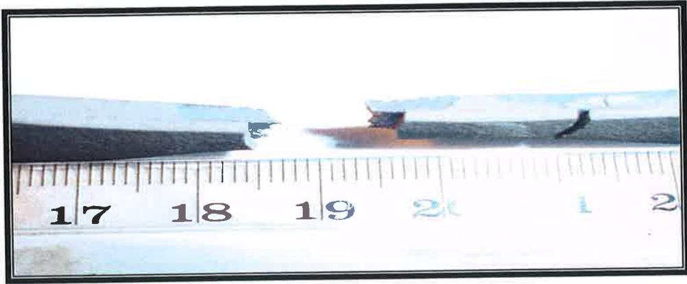
Figure B49: Welded Carbon steel specimen 5 mm size in as received (no exposure) condition tensile tested.
