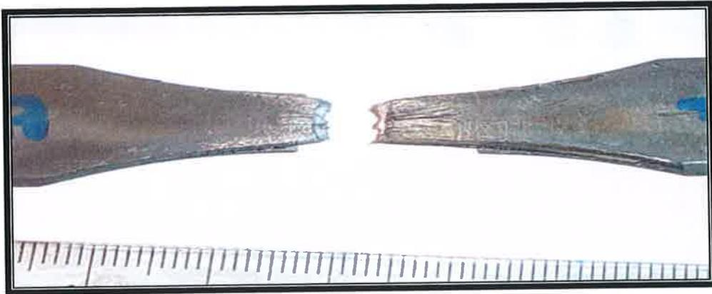
Figure B28: Welded stainless steel 5 mm size after three (3) week exposure to brine solution tensile tested.
