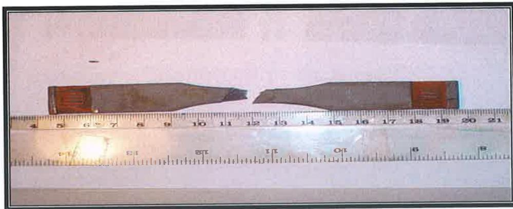
Figure B60: Carbon steel specimen after three (3) weeks exposure to brine solution tensile tested.
