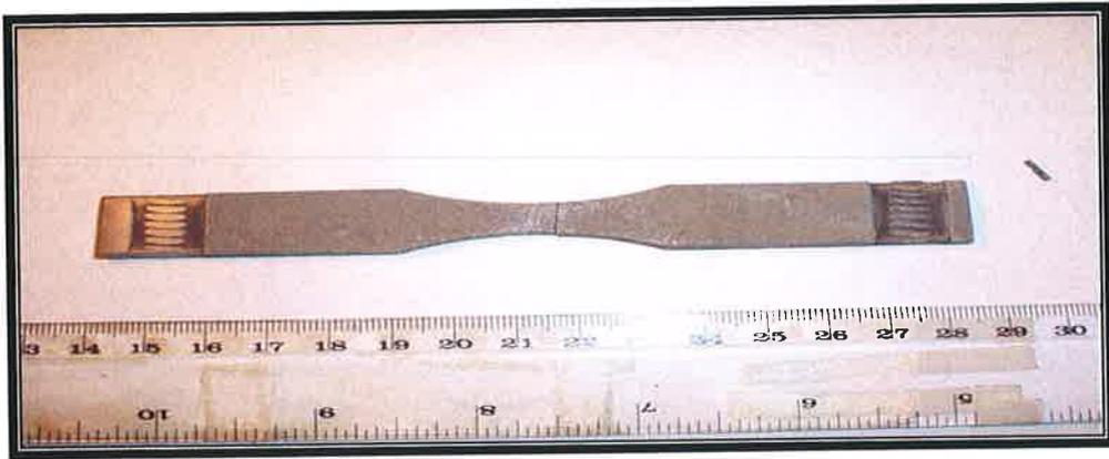
Figure B76: Stainless steel specimen after three (3) weeks exposure to brine solution fatigue tested.
