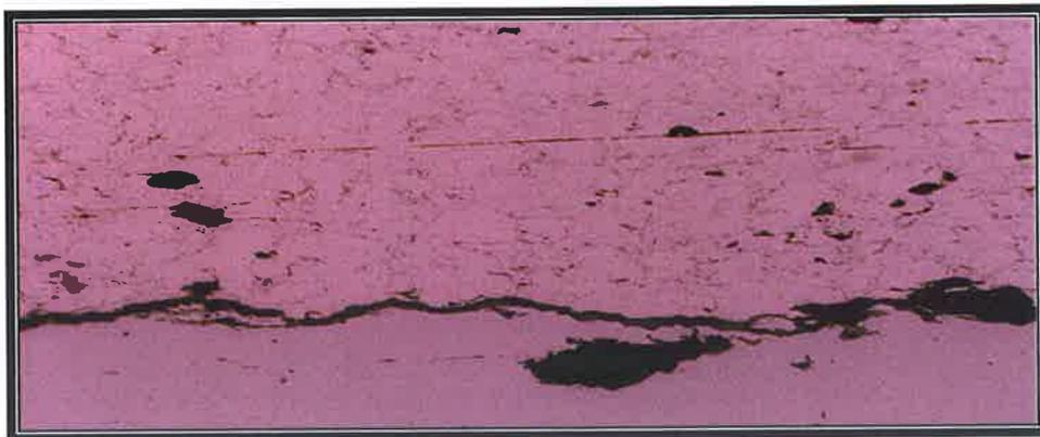
Figure A6: Carbon Steel after one (1) week exposure to brine solution and tensile tested.
