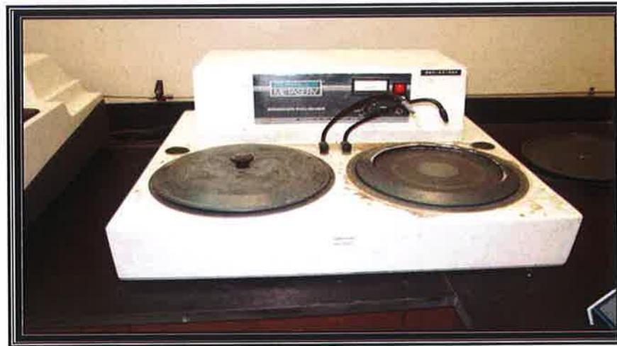
Figure 9: Grinding equipment used to grind and polish all specimens.
