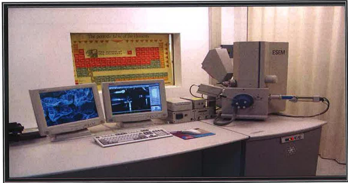
Figure 10: ESEM/EDS facility used for coating characterization (Philips XL-30).
