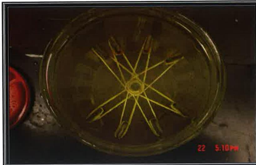
Figure 23: 3 liters, Glass-container test vessel containing 3.5 % sodium chloride.
