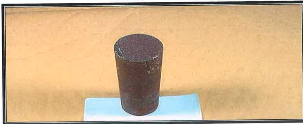
Figure B3: Carbon Steel round solid specimen tensile tested post brine solution exposure: Side view.
