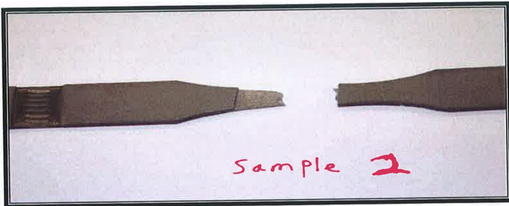
Figure B11: Stainless Steel specimen after one (1) week exposure to brine solution tensile tested.
