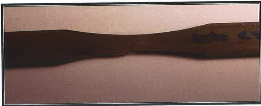
Figure B48: Welded Carbon steel specimen 5 mm size after three (3) weeks exposure to brine solution prior to mechanical testing.
