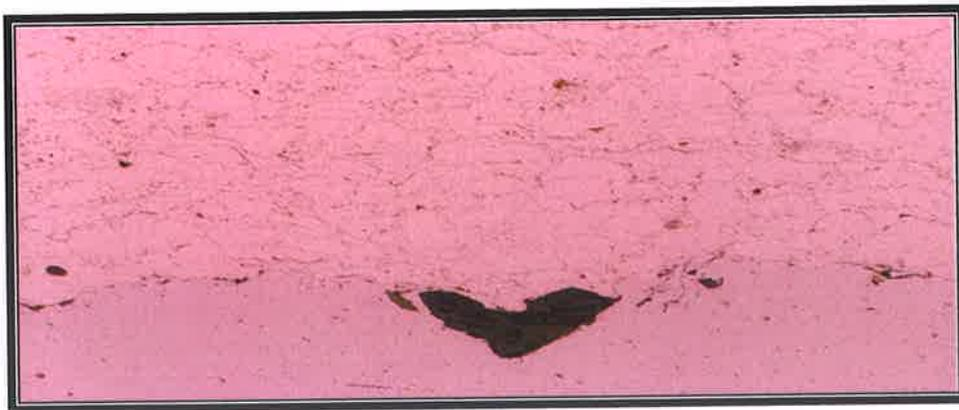
Figure A81: Carbon Steel after one (1) week exposure to brine solution tensile tested.
