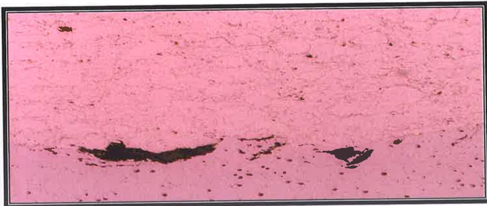
Figure A78: Carbon Steel after one (1) week exposure to brine solution tensile tested.
