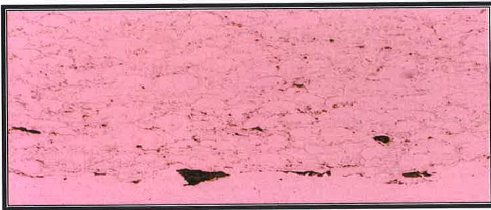
Figure A68: Stainless Steel after three (3) week exposure to brine solution fatigue tested.
