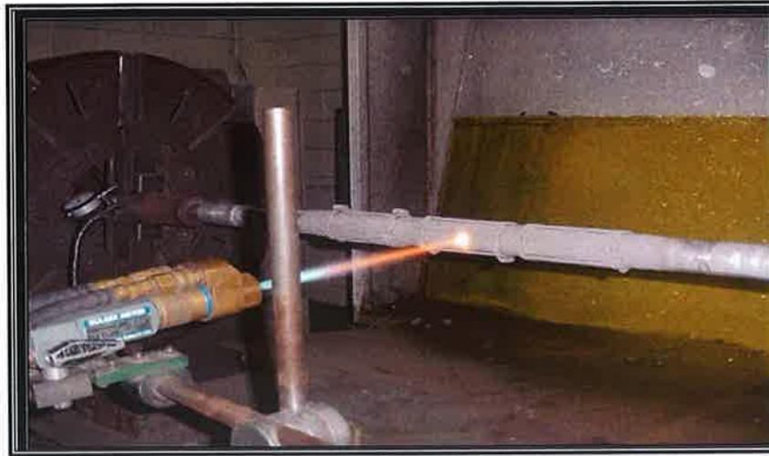
Figure 19: Flat specimens being sprayed using the gun traverse unit on a moving table
