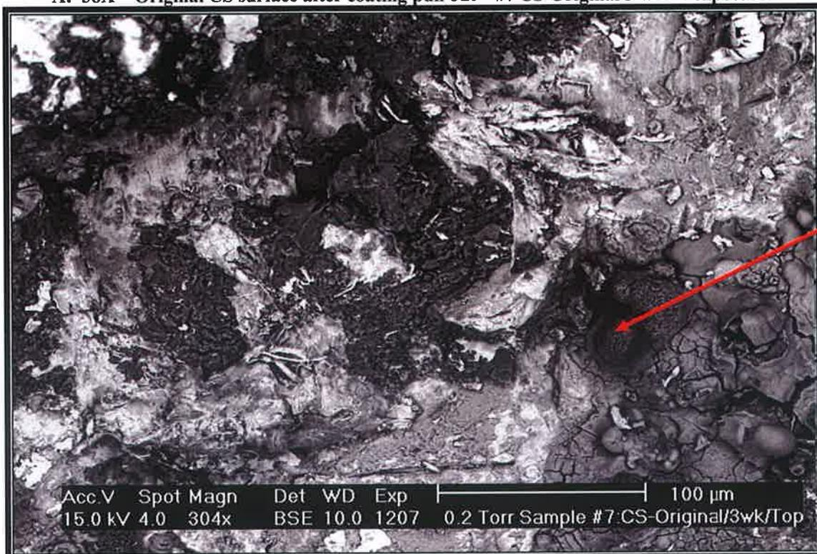
**B: 304X Original CS surface after coating pull out #7 CS-Original 3 weeks exposure.**
