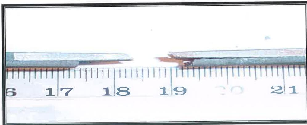
Figure B36: Stainless steel specimen after three (3) weeks exposure to brine solution tensile tested.
