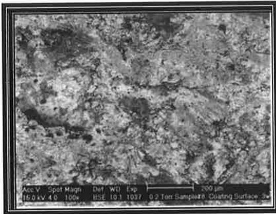
Coating remained on top surface of carbon steel dummy after three weeks exposure to brine solution.
