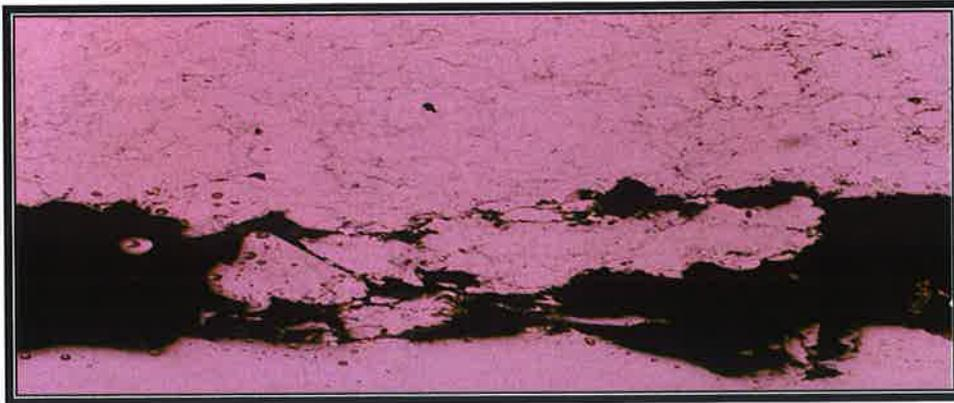
Figure A19: Stainless Steel after one (1) week exposure to brine solution tensile tested.
