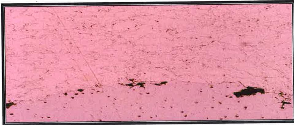
Figure A79: Carbon Steel after one (1) week exposure to brine solution tensile tested.
