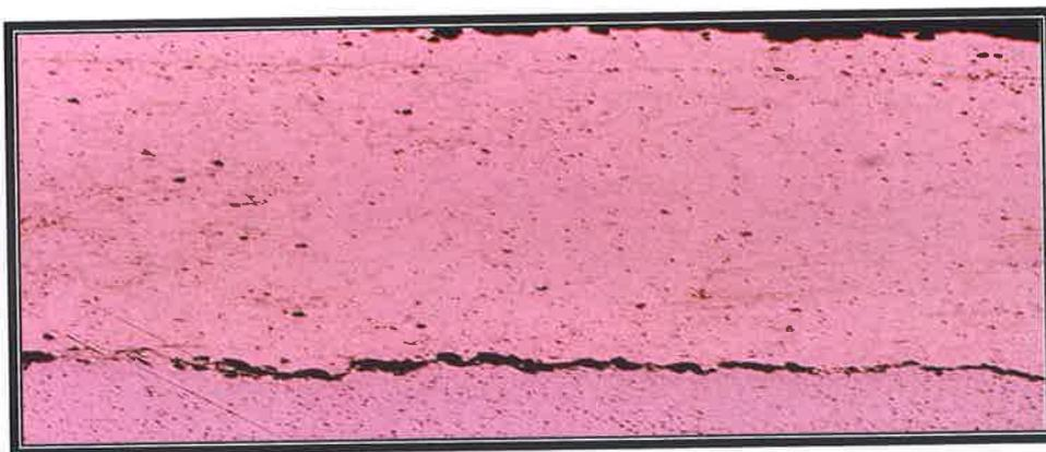
Figure A105: Carbon Steel after three (3) weeks exposure to brine solution tensile tested.
