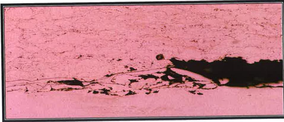
Figure A121: Stainless Steel after one (1) week exposure to brine solution tensile tested.
