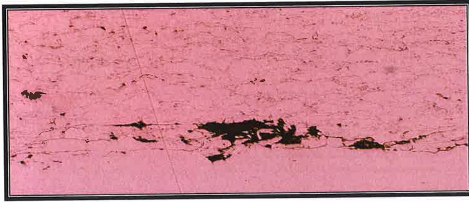
Figure A118: Stainless Steel after one (1) week exposure to brine solution tensile tested.
