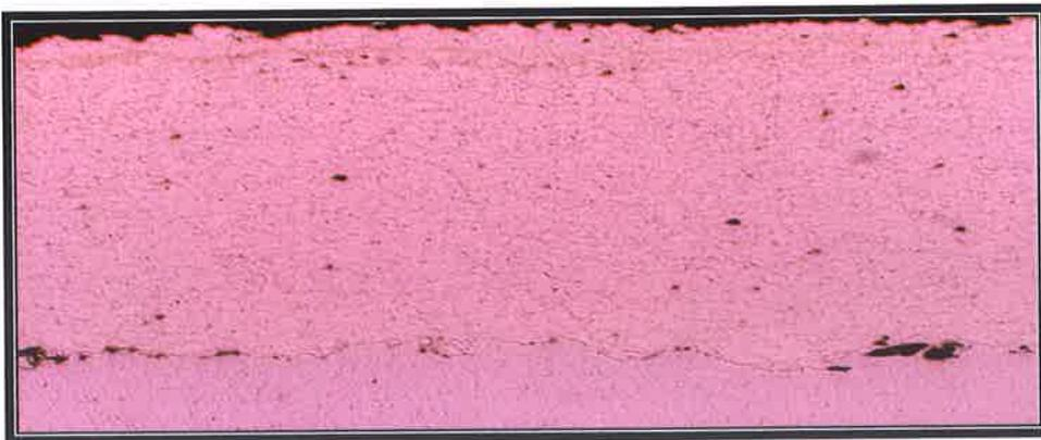
Figure A72: Carbon Steel after one (1) week exposure to brine solution tensile tested.
