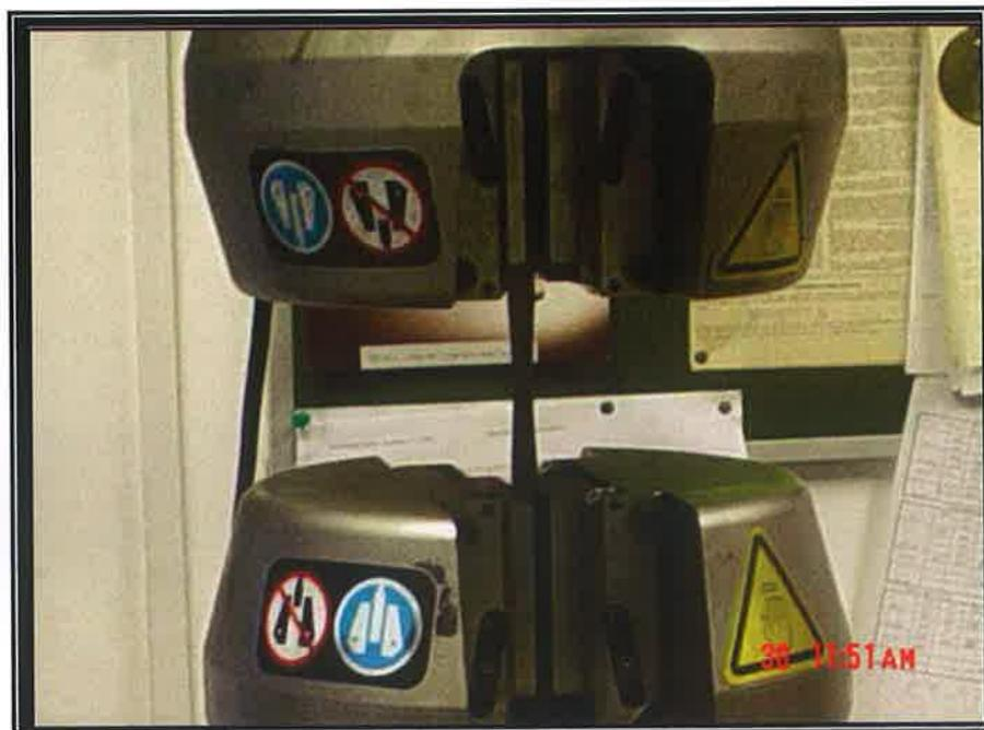
Figure 22: Flat sheet specimen fitted to the fixture ready for tensile testing.
