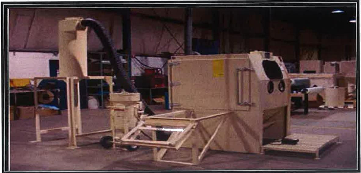
Figure 3: Grit blasting facility, Courtesy of [190].
