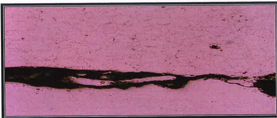
Figure A17: Stainless Steel after one (1) week exposure to brine solution tensile tested.
