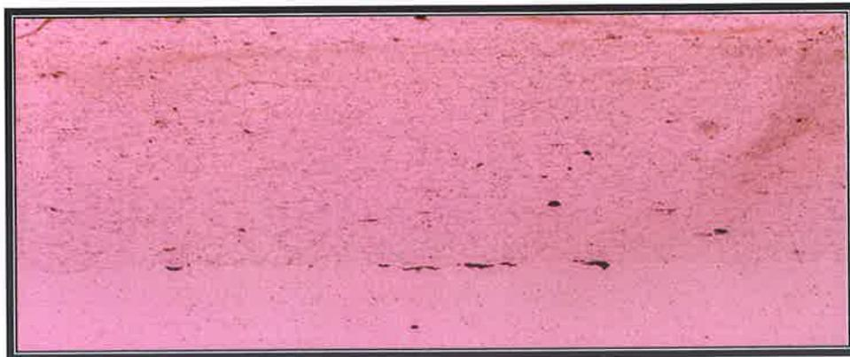
Figure A63: Stainless Steel after three (3) week exposure to brine solution fatigue tested.
