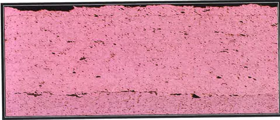
Figure A106: Carbon Steel after three (3) weeks exposure to brine solution tensile tested.
