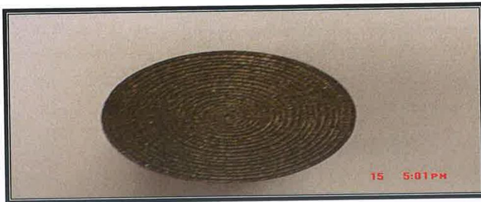
Figure B6: Stainless Steel round solid specimen after two (2) weeks exposure to brine solution tensile tested: Top view.
