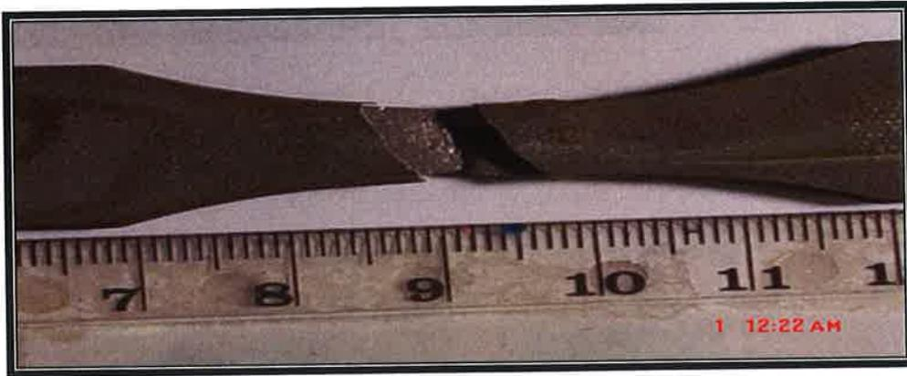
Figure B22: Welded stainless steel 3 mm size after three (3) weeks exposure to brine solution tensile tested.
