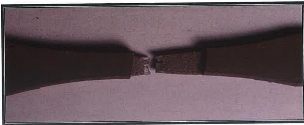
Figure B33: Stainless steel specimen after three (3) weeks exposure to brine solution tensile tested.
