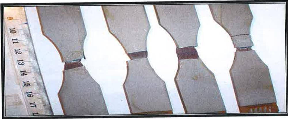
Figure B52: Carbon steel specimens after one (1) week exposure to brine solution tensile tested.
