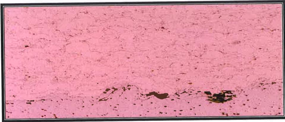
Figure A77: Carbon Steel after one (1) week exposure to brine solution tensile tested.
