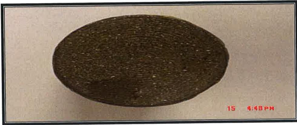
Figure B7: Stainless Steel round solid specimen after three (3) weeks exposure to brine solution tensile tested: Top view.
