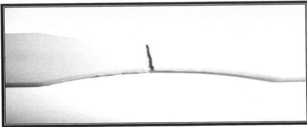
Figure B68: Welded Carbon steel specimen 5 mm size in as received condition (no exposure) fatigue tested.
