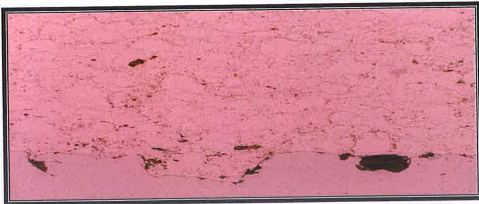
Figure A90: Carbon Steel after one (1) week exposure to brine solution fatigue tested.
