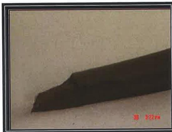
Figure 54: A photograph showing coated carbon steel specimen post 3 weeks static corrosion exposure after fatigue failure. Peeling-off coating from the base material is evident.
