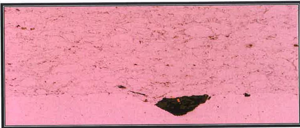
Figure A71: Stainless Steel after three (3) week exposure to brine solution fatigue tested.
