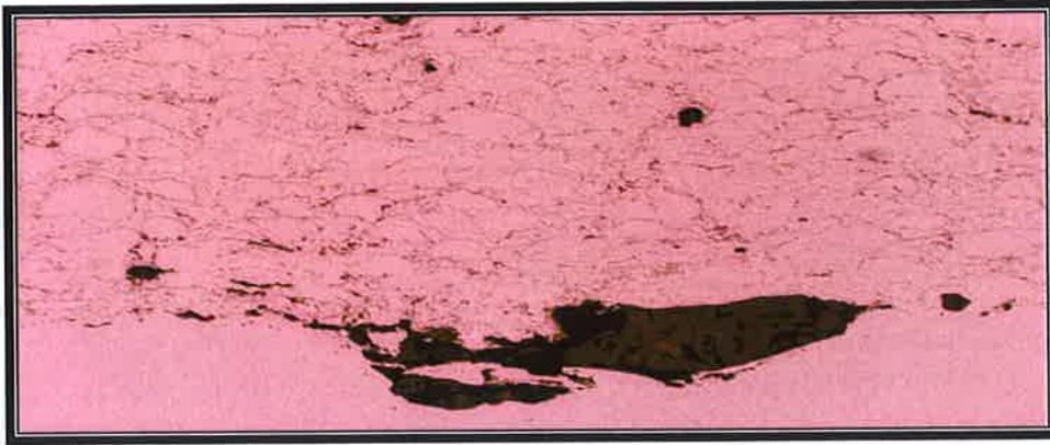
Figure A58: Stainless Steel after one (1) week exposure to brine solution fatigue tested.
