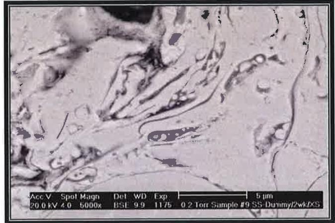
B: 5000X Coating Cross section on Dummy-SS after two weeks exposure to brine solution.
