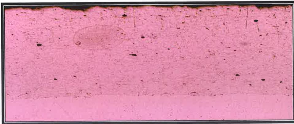
Figure A66: Stainless Steel after three (3) week exposure to brine solution fatigue tested.
