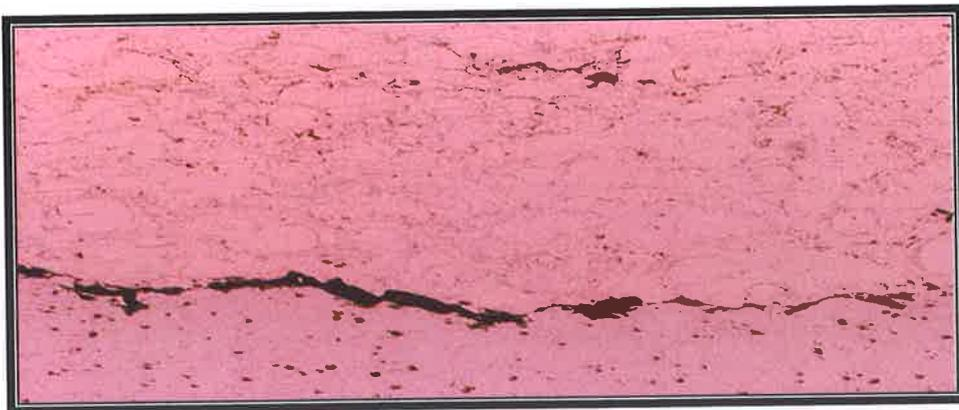
Figure A108: Carbon Steel after three (3) weeks exposure to brine solution tensile tested.
