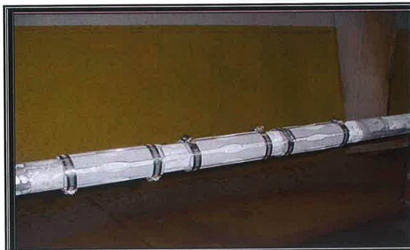
Figure 18: Flat specimens after been sprayed onto the mandrel left to cool.
