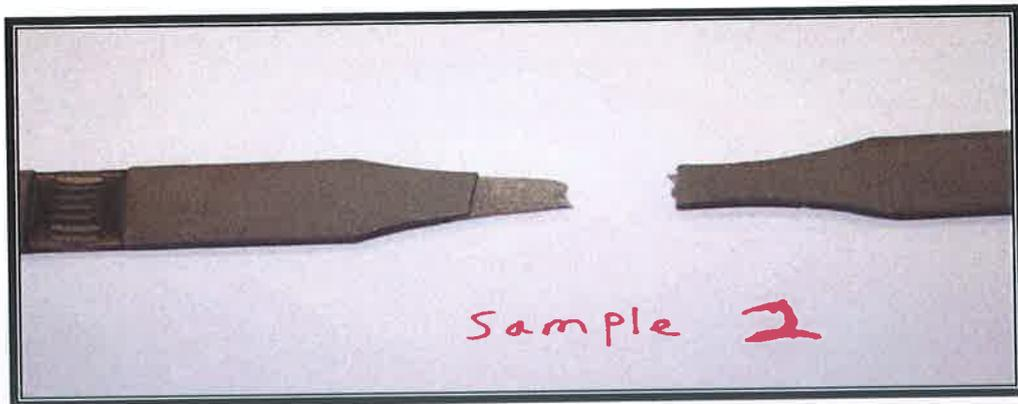
Figure B12: Stainless Steel specimen after one (1) week exposure to brine solution tensile tested.
