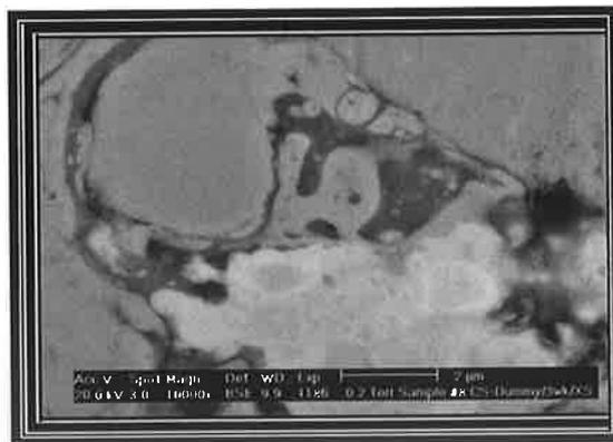
Coating cross-section on a carbon steel dummy after three weeks exposure to brine solution.
