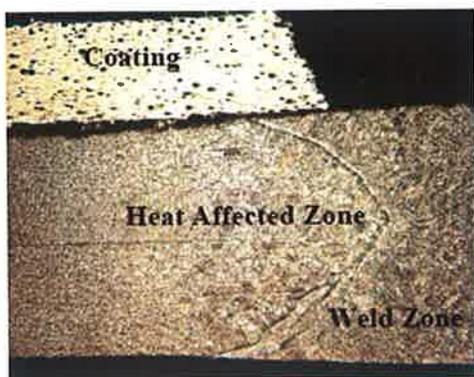
Coating is peeled off from the weld surface.
