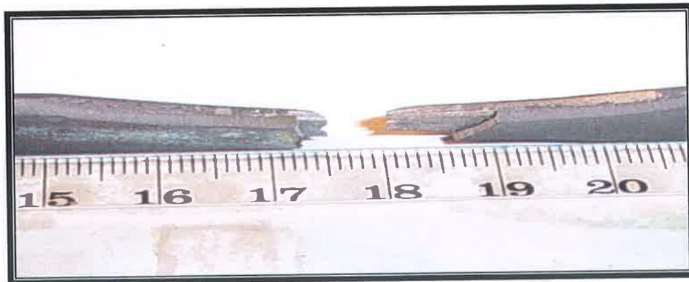
Figure B27: Welded stainless steel 5 mm size after three (3) week exposure to brine solution tensile tested.
