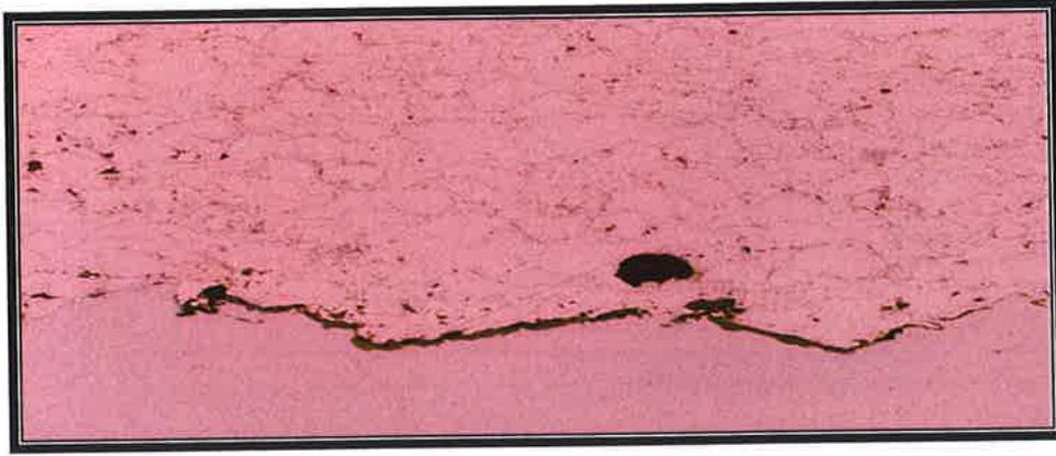
Figure A88: Carbon Steel after one (1) week exposure to brine solution fatigue tested.
