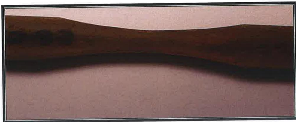
Figure B42: Welded Carbon steel specimen 2.5 mm size after three (3) weeks exposure to brine solution prior to mechanical testing.
