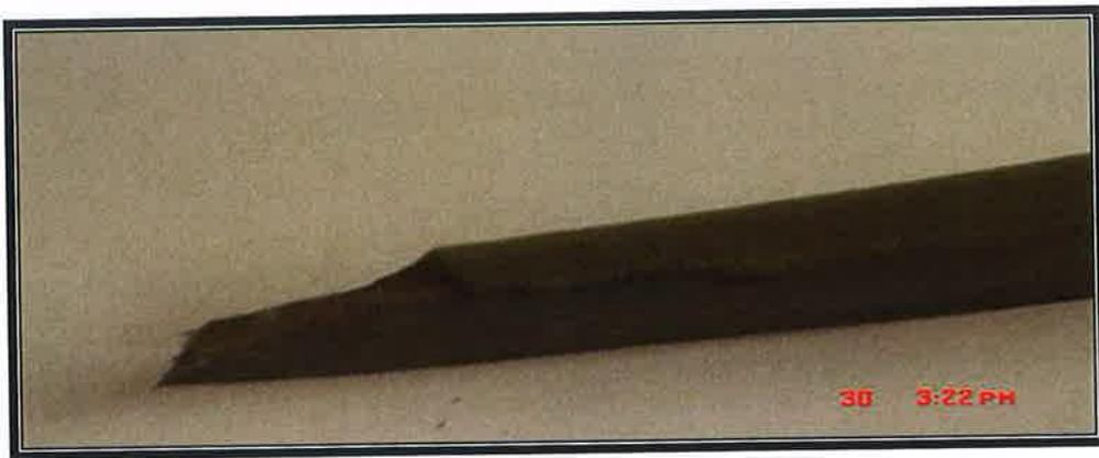
Figure B17: Carbon Steel Specimen after one (1) week exposure to brine solution tensile tested.
