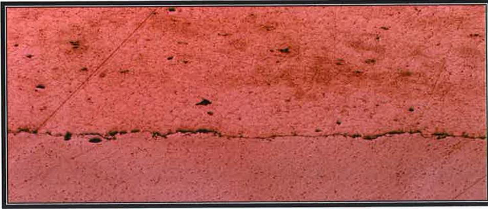
Figure A22: Carbon Steel after one (1) week exposure to brine solution tensile tested.
