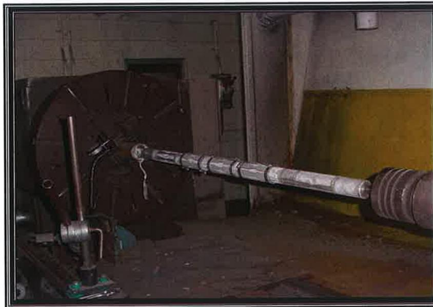
Figure 12: Pre-heated treated for flat sheet substrates mounted onto mandrel.
