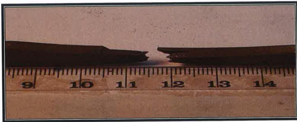
Figure B59: Carbon steel specimen after three (3) weeks exposure to brine solution tensile tested.
