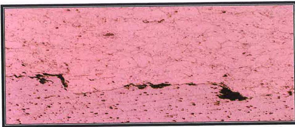
Figure A107: Carbon Steel after three (3) weeks exposure to brine solution tensile tested.
