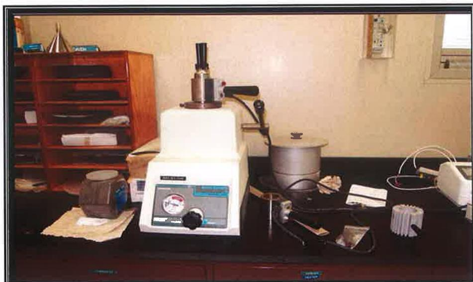
Figure 8: A mounting apparatus used for specimen's mounting.
