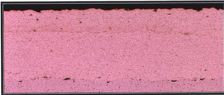
Figure A74: Carbon Steel after one (1) week exposure to brine solution tensile tested.
