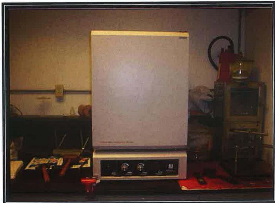
Figure 5: A view of the oven and its set-up used to cure the adhesive.
