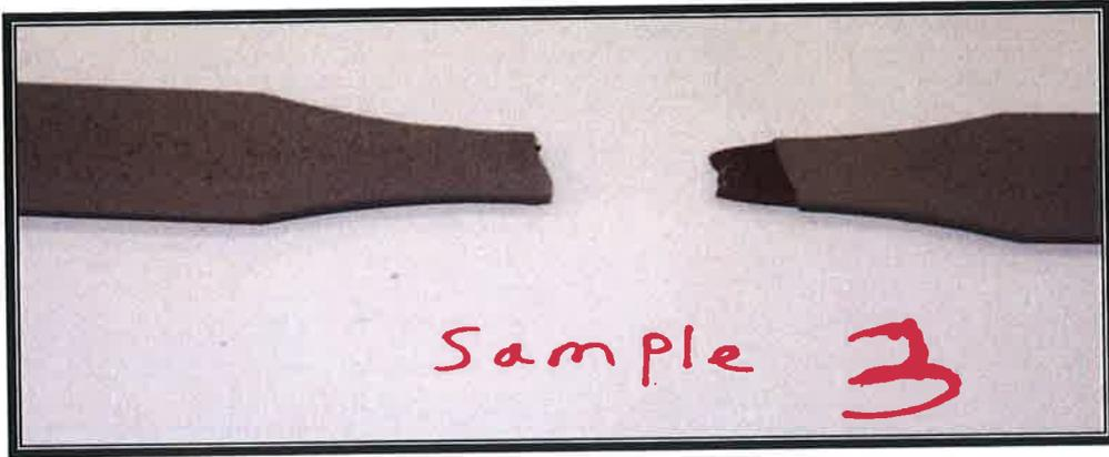
Figure B13: Carbon Steel specimen after one (1) week exposure tensile tested.
