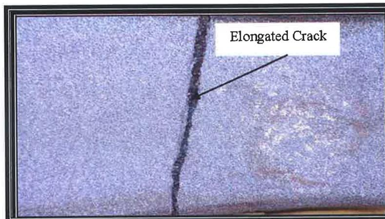
Figure 47 - Micrograph of a crack site in HVOF coating (15X magnification).
