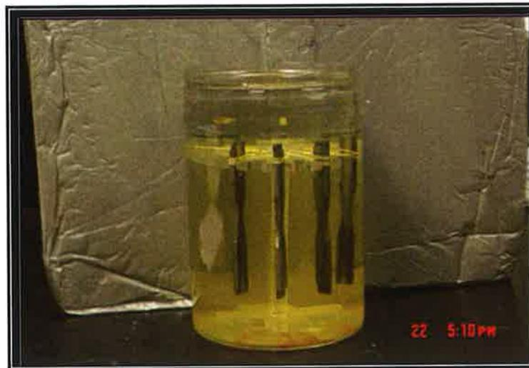
Figure 24: coated specimens fully immersed with equal separation within 3.5 % NaCl.
