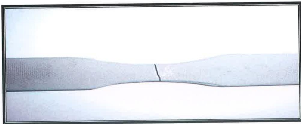
Figure B72: Carbon steel specimen in as received condition (no exposure) fatigue tested.
