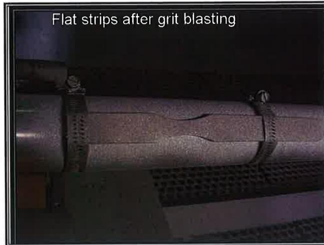
Figure 11: Grit blasted substrate ready for pre-heat treatment.
