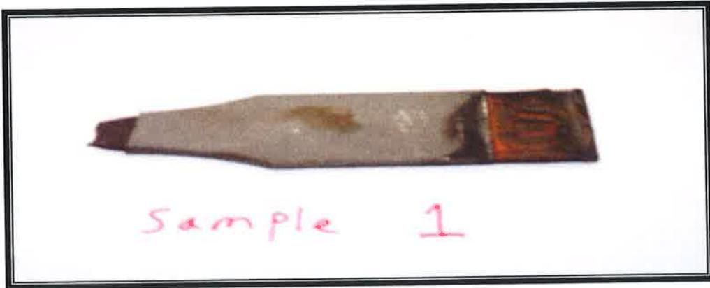
Figure B10: Carbon Steel specimen after one (1) week exposure to brine solution tensile tested.
