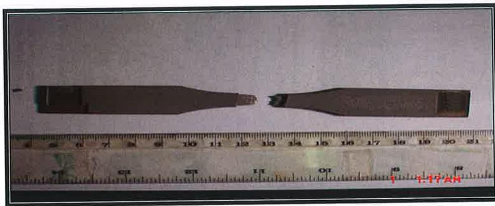
Figure B29: Welded stainless steel 5 mm in as received condition (no exposure) tensile tested.
