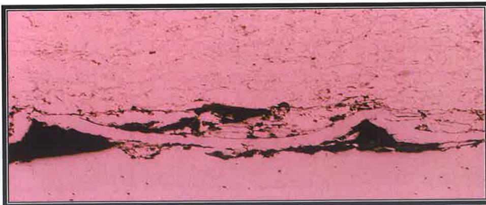
Figure A51: Stainless Steel after one (1) week exposure to brine solution tensile tested.
