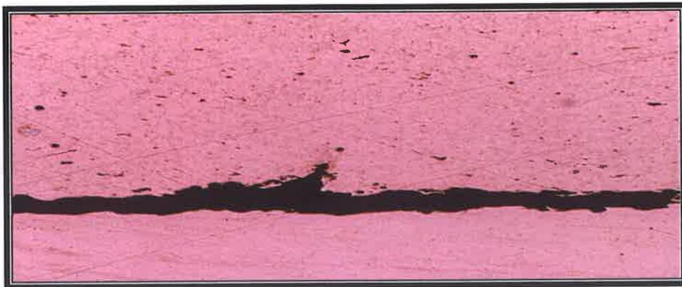
Figure A33: Stainless Steel after three (3) weeks exposure to brine solution tensile tested.
