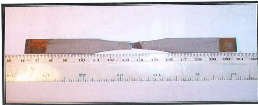
Figure B57: Carbon steel specimen after one (1) week exposure to brine solution tensile tested.
