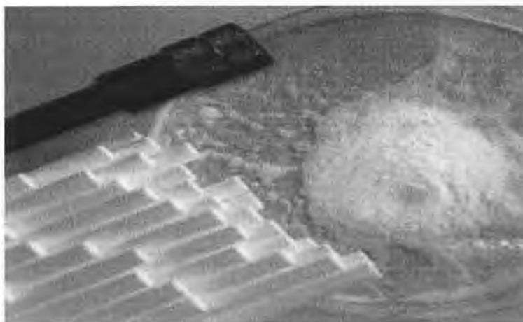
Figure 1.8: (a) shows the total number of papers published on monolithic columns for HPLC during the time period 1989-2003 [60] and (b) monolithic silica rods (before and after cladding) compared to particulate type silica used in conventional HPLC silica columns [62].
