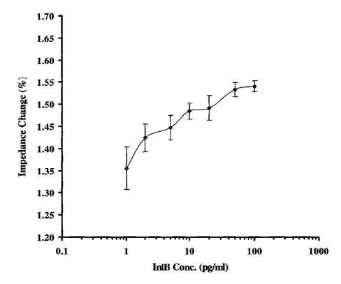
**Figure 5.21** Calibration profile showing percentage impedance response against InlB concentrations (1-100 pg/ml) for anti-InlB-doped PANI-coated electrodes at 1Hz. Error bars are calculated from the standard deviations of the mean value of three replicates on two separate electrodes (six replicates in total).
