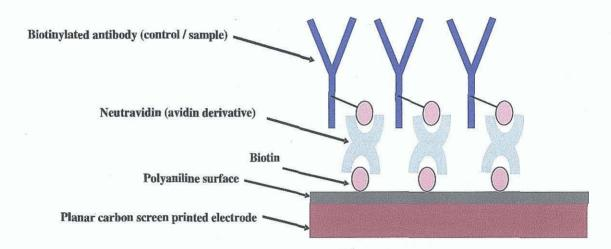
**Figure 5.5** Schematic representation of biomolecule immobilisation onto polyaniline (PANI) sensor surfaces via biotin-avidin coupling. Biotinylated antibodies, both sample (anti-InIB antibody) and control (anti-IgG antibody) were specifically coupled to the biotinylated polymer (polyaniline) films using the avidin derivative neutravidin, which formed avidin-biotin bridges. This method allowed controlled immobilisation of biomolecules at the sensor surface.
