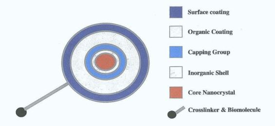
**Figure 1.8** Schematic depicting the component layers of a quantum dot. An inorganic zinc sulphide (ZnS) shell encapsulates the core nanocrystal composed of cadmium selenide (CdSe). The inorganic shell is subsequently capped and an organic layer and a polymer surface coating are applied to enable biomolecule attachment. For the quantum dots used in this thesis the polymer shell is directly coupled to streptavidin through a carbodiimide-mediated coupling reaction for biomolecule attachment.
