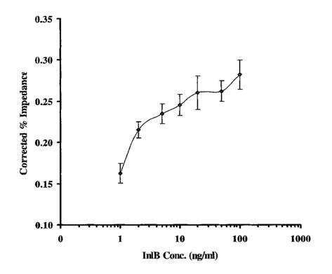
**Figure 5.19** Corrected calibration curve showing the percentage impedance change from the baseline trace for increasing InlB antigen concentrations, at a frequency of 1Hz (5mV a.c). Error bars are calculated from the standard deviations of the mean value of three replicates on two separate electrodes (six replicates in total).
