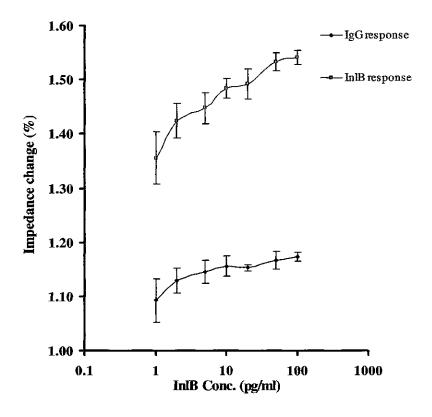
**Figure 5.22** Calibration curve showing the percentage impedance change from the baseline trace for increasing InlB antigen concentrations, at a frequency of 1Hz (5mV AC) for both sample and control doped sensors in the picogram range. Error bars are calculated from the standard deviations of the mean value of three replicates on two separate electrodes (six replicates in total).
