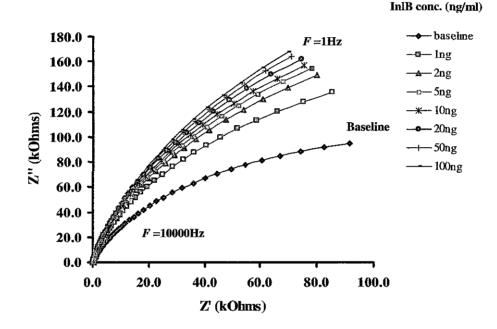
**Figure 5.7** Nyquist plot showing the faradaic component (Z') against the capacitive component (Z'') for anti-InlB-doped PANI-films on carbon electrodes, following exposure to various concentrations of InlB (1-100ng/ml).
