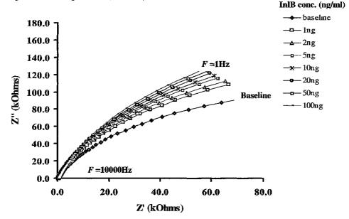
**Figure 5.17** Nyquist plot showing the faradaic component (Z') against the capacitive component (Z'') for PANI-films on carbon electrodes, containing no antibody, following exposure to various concentrations of InlB (1-100ng/ml).
