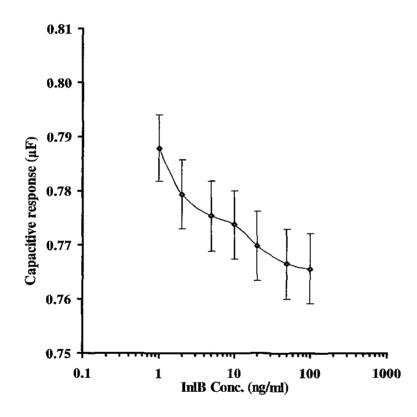
**Figure 5.12** Calibration curve of the non-faradaic capacitive response against InlB concentration (ng/ml) for anti-InlB-doped PANI-coated carbon electrodes at the characteristic frequency of 28Hz. The characteristic frequency is the frequency where the phase angle is closest to 90°. Error bars are calculated from the standard deviations of the mean value of three replicates on two separate electrodes (six replicates in total).
