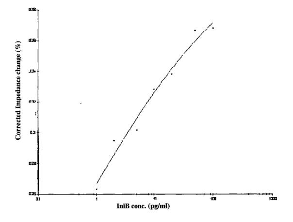
**Figure 5.23b** Calibration curve showing the corrected response of the system for InlB detection. The data were fitted to 4-parameter equation using Biaevaluation software, for calculation of lower limit of detection using the 3 sigma method. The curve displays total impedance (Z) against InlB concentration. The lower limit of detection (LOD) is equal to 4.1pg/ml
