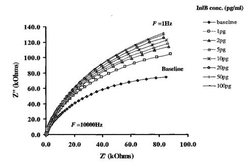
**Figure 5.20** Nyquist plot showing the faradaic component (Z') against the capacitive component (Z'') for anti-InlB-doped (sample) PANI-films on carbon electrodes, following exposure to various concentrations of InlB (1-100pg/ml).
