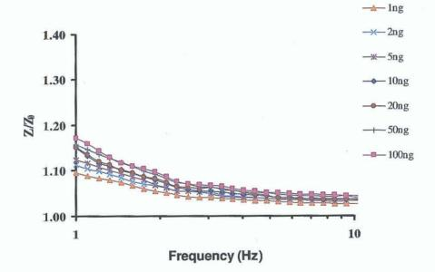
**Figure 5.14** Bode plot showing the faradaic and non-faradaic changes in total impedance for anti-IgG-doped PANI-films on carbon electrodes following exposure to various concentrations of InIB, normalised from the baseline trace  $(Z/Z_0)$ .
