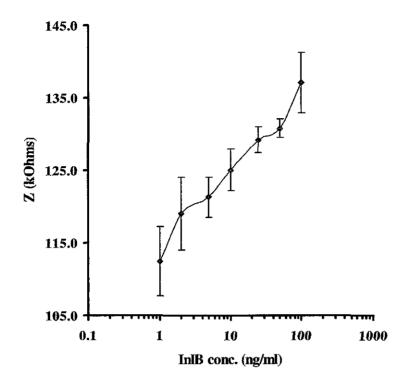
**Figure 5.6** Calibration curve of InlB concentration at 1Hz. The calibration curve was generated as a result of exposure of an anti-InlB loaded PANI-film to increasing concentrations of InlB (1-100ng/ml). The curve displays total impedance (Z) against InlB concentration (ng/ml). Error bars are calculated from the standard deviations of the mean value of three replicates on two separate electrodes and CVs of less than 5% were found.
