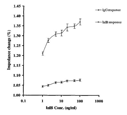
**Figure 5.18** Calibration curve showing the percentage impedance change from the baseline trace for increasing InlB antigen concentrations, at a frequency of 1Hz (5mV a.c) for both sample (InlB response) and control (IgG response) sensors. Error bars are calculated from the standard deviations of the mean value of three replicates on two separate electrodes (six replicates in total).
