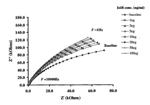
**Figure 5.13** Nyquist plot showing the faradaic component (Z') against the capacitive component (Z'') for anti-IgG-doped (control) PANI-films on carbon electrodes, following exposure to various concentrations of InlB (1-100ng/ml).
