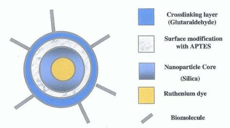
**Figure 1.10** Schematic depicting the component layers of ruthenium dye-doped silica nanoparticles. A silica shell encapsulates the constituent dye (ruthenium) using a water in oil microemulsion technique. The silica surface of the doped nanoparticles is modified for biomolecule attachment by silanisation with aminopropyltrimethoxysilane (APTES) and subsequent glutaraldehyde crosslinking.
