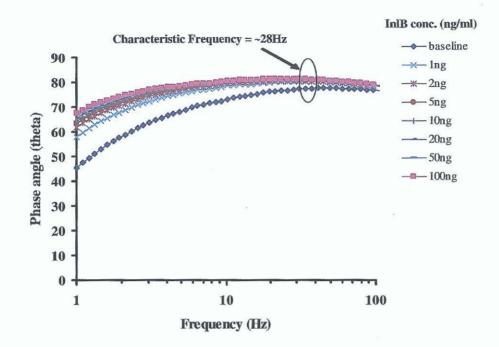
**Figure 5.11** *Plot showing frequency vs. phase angle for each concentration of InlB* (1-100ng/ml). The characteristic frequency, where the phase angle is closest to 90° was determined to be approximately 28 Hz.
