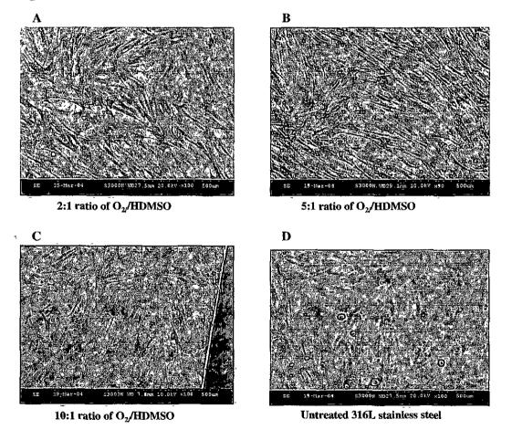
**Figure A3** SEM images of stainless steel substrates post incubation in culture with varying ratios of HDMSO/O<sub>2</sub>. Cell adhesion and proliferation is greatest on the films with lowest ratio of oxygen to HDMSO (2:1). Higher magnification and examination of a greater sample set would give more detail as to the actual effect of the thin film on the stainless steel substrates.
