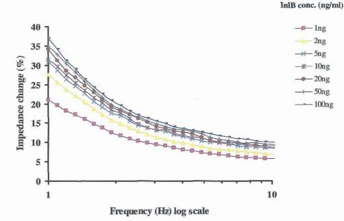
**Figure 5.9** Percentage impedance change from the baseline trace for increasing InlB antigen concentrations (1-100ng/ml), in the frequency range 1- 10Hz, for InlB sensors. The percentage impedance change increases for increasing InlB antigen concentrations between 1-10Hz.
