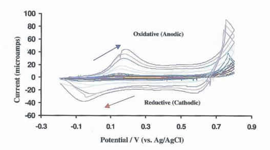
**Figure 5.3** Cyclic voltammogram showing the potentiodynamic electrodeposition of polyaniline (PANI) as a thin-film on planar carbon screen-printed electrodes. The working electrode potential was scanned from -200mV to 800mV (vs. Ag/AgCl) and peak increases in anodic and cathodic current transients were recorded.
