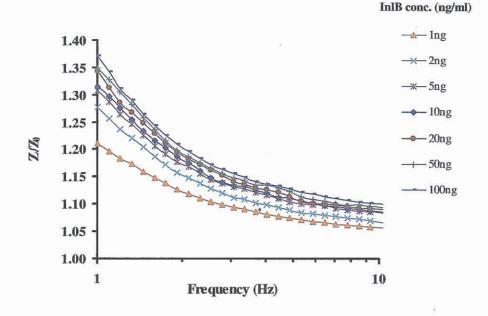
**Figure 5.8** Bode plot showing the faradaic and non-faradaic changes in total impedance for anti-InlB-doped PANI-films on carbon electrodes following exposure to various concentrations of InlB, normalised from baseline trace  $(Z/Z_0)$ .
