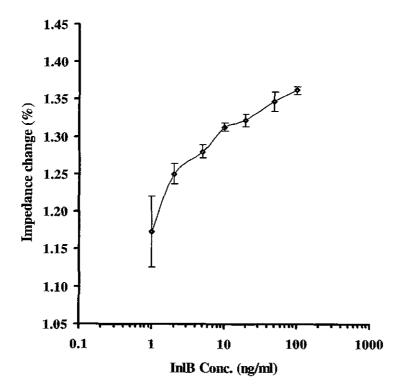
Figure 5.10 Calibration curve of InlB concentration at 1Hz. The curve was generated as a result of exposure of anti-InlB-loaded PANI-films to increasing concentrations of InlB at 1 Hz. The curve displays the percentage change in impedance for each InlB concentration (ng/ml), normalised against the baseline response (zero antigen). Error bars are calculated from the standard deviations of the mean value of three replicates on two separate electrodes (six replicates in total).
