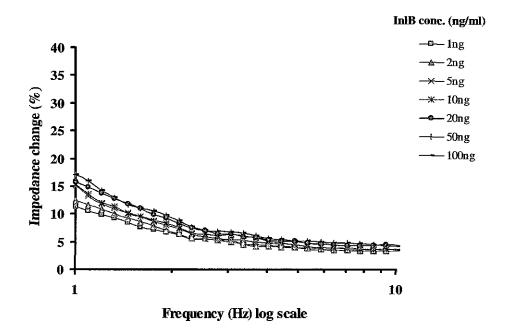
**Figure 5.15** Percentage impedance change from the baseline trace for increasing InlB antigen concentration in the frequency range 1-10Hz, for IgG (control) sensors. The percentage impedance change increases for increasing InlB antigen concentrations, between 1-10Hz. However, the overall increase in impedance is low (<8%).
