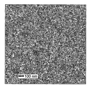
Figure 4.22 Transmission electron microscopy (TEM) micrograph of the high brightness ruthenium dye-doped nanoparticles with protecting groups THPMP and APTES added. The average particle size was calculated as 77.9nm  $\pm 5.09$  nm (Scale = 100nm).
