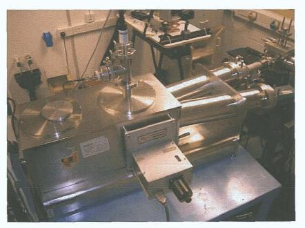
Figure 10: ARC VM-521 Spectrometer
