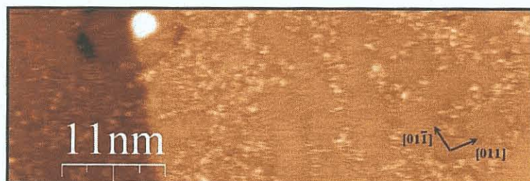
Figure 4.2: The TMA modulated row structure surrounded by disordered TMA molecules at a coverage of 8.1 \times 10^{-3}L . V_s = -0.75 V, I_t = 0.5 nA, 54.7 \times 18.3 nm.
