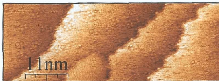
Figure 4.3: STM image of the TMA quad structure which always aligns with the substrate along the [011] and [01\bar{1}] directions, V_s = 1.0 V, I_t = 0.5 nA, 54.8 \times 20.2 nm.
