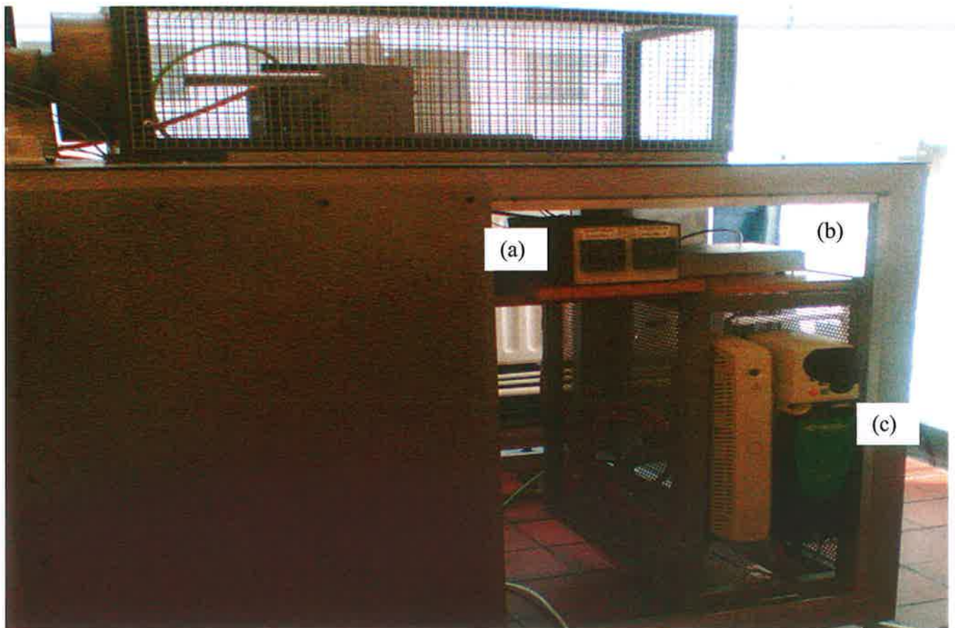
Figure 2.29 Picture of (a) temperature controller, (b) National Instrument data acquisition box and (c) motor controller.
