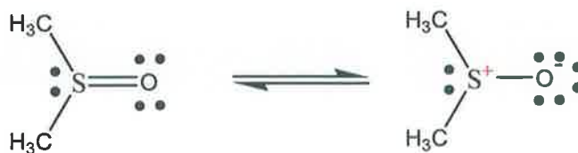
Scheme 2.3. DMSO molecule at equilibrium with the partial negative formal charge on oxygen and partial positive charge on sulfur.
