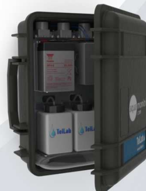
TellLabs Aqua Monitrix System (Targets: Nitrate, Nitrite, pH, Chemical Oxygen Demand)
