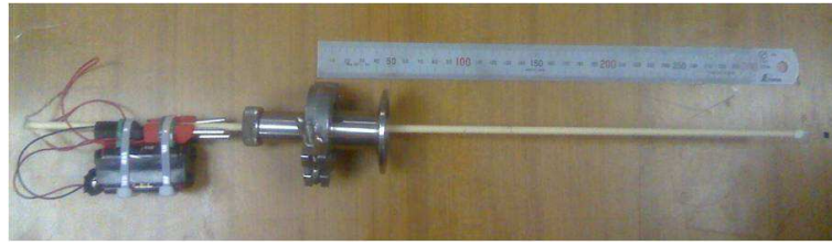
Figure 4.8: Hall probe for the measurement of magnetic field strength.
