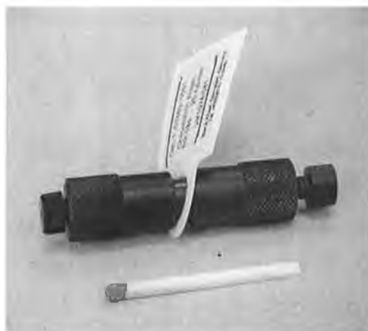
Figure 7-1. Short 2.5 cm monolithic ODS column. Merck Chromolith Flash RP-18e 25 mm X 4.6 mm column.
