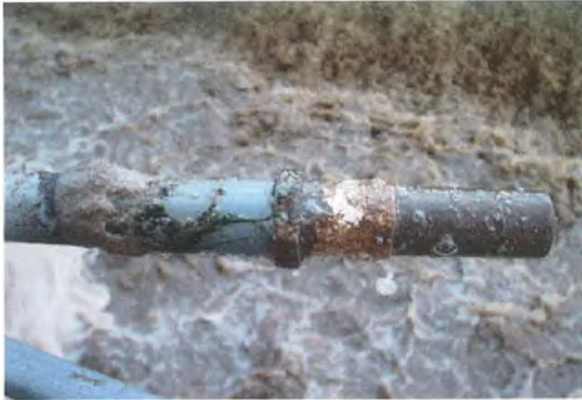
Figure 5.13: Phase 1 Field Testing of DO Waste-Water Monitoring Probe.
