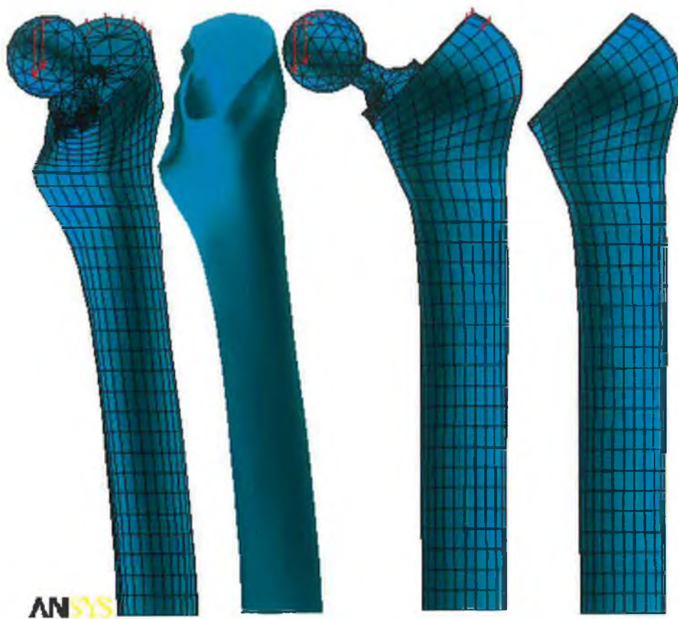
Figure 4.16: Finite element modelling of the treated femur.
