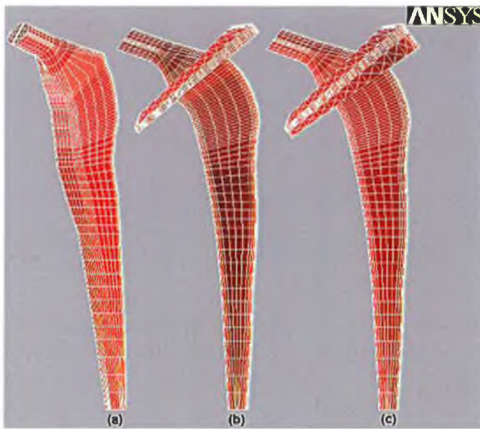
Figure 6.3: 3-D finite element meshes of hip prosthesis. (a) Collarless cemented hip prosthesis, (b) Collared cemented hip prosthesis without skirt and damper, and (c) Skirt-Collared cemented hip prosthesis provided with a damper.
