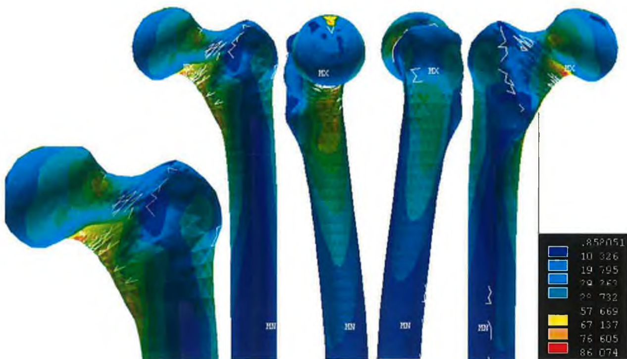
Figure 4.15: The Von Mises proximal femur stress contours shows maximum stresses/strains are located in the proximal neck region.
