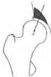
Figure 1.32: Triangular stress diagram in a hip joint with laterally shifted force R . [202]
