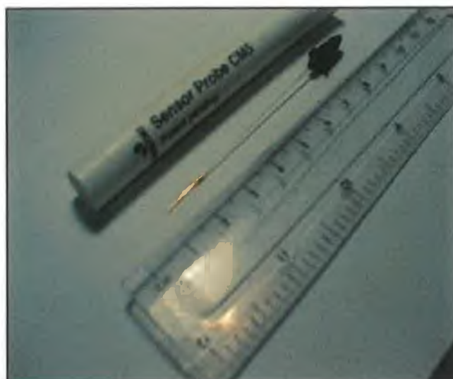
Figure 5.2 : The BIAProbe. A small thin fibre optic that has had one end coated with a gold layer. This is the sensing end of the probe. It is immersed and the signal is passed from the probe to a data acquisition device. Binding is detected using a combination of the light passed through the fibre optic and SPR.
