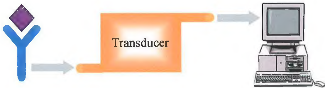
Figure 1.10 : Schematic representation of the principle of a biosensor. An event occurs that creates a change in the system, e.g. an antibody binding to an antigen. The signal is then fed to the transducer. A transducer is an instrument that changes a signal into a form compatible with a data processing device. The transducer senses that change and converts it into a signal. The altered signal is then passed to a data processing unit for handling, storage and display.
