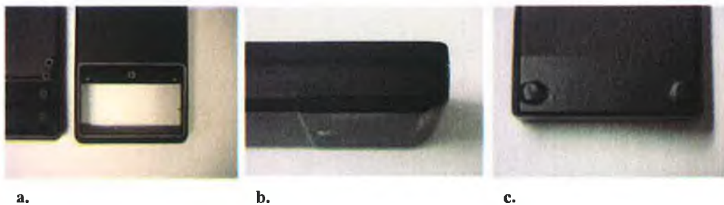
Figure 2-4 Illustrates complete sealing of the Datec-Pocket boxes (6.5 × 12.0 × 2.2 cm) a. OKW enclosure with seal b. silicon used to completely seal the box c. tape ensures maximum protection
