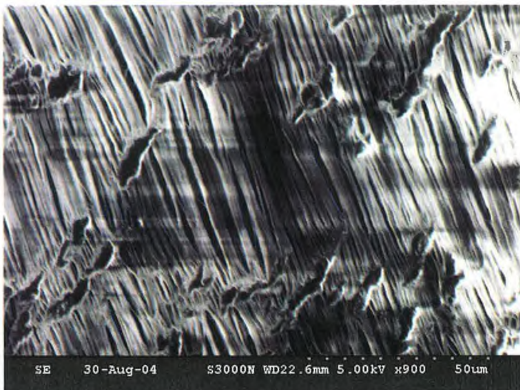
Figure 6-5 PTFE membrane in its original form (Magnification \times 900 )
