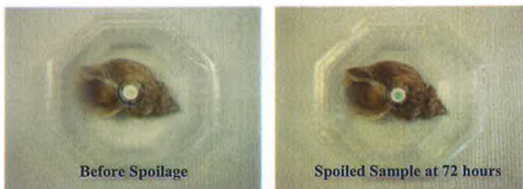
Figure 4-15 Sensor spot before and after spoilage
