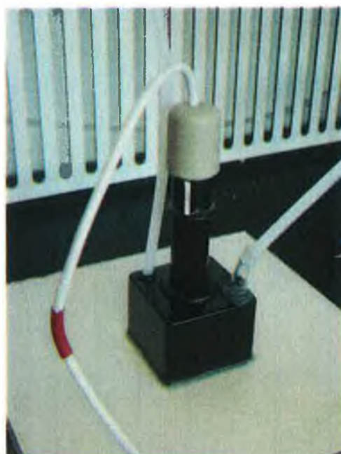
Figure 4-13 Experimental set-up for sensor calibration using ammonia gas. Mass flow controllers enabled known concentrations of ammonia gas to be delivered to the flow-cell by mixing different proportions of pure nitrogen (maximum flow rate 100\text{-}900\text{cm}^3\text{ min}^{-1} ) and 0.01% ammonia in nitrogen (maximum flow rate 50\text{cm}^3\text{ min}^{-1} ). The pure nitrogen was allowed to flow through a humidifier before it was mixed with 0.01% ammonia in nitrogen. The gas mixture entered the flow cell through the inlet tube where it reacted with the sensor.
