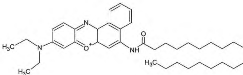
Figure 4-2 Polymer/plasticiser-soluble pH indicator (Octadecyl Nile Blue)
