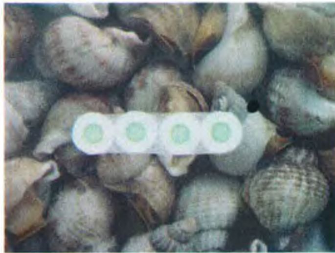
Figure 6-7 Digital images of sensors representing cooked whelk samples stored at room temperature (bottom) and in the fridge (top) taken at 14 hours. The sensors representing the room temperature samples are green (bottom) whereas the sensors representing the fridge samples are greenish-yellow (top). According to the microbial data and TVB-N values, at 14 hours the room temperature samples are ‘gone off’ while the fridge samples are ‘going off’. The colour of the sensors can be used as a crude indication of the on-set of spoilage.
