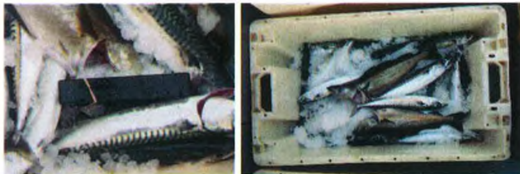
Figure 3-18 RF Temperature logger 2 placed in a box of mackerel (partially iced)
