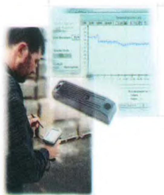
Figure 1-9 The i-Q32T system (50). A handheld device allows the temperature data to be accessed via radio frequency communications.
