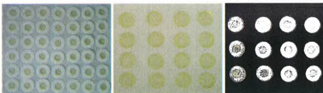
Figure 4-9 Digital images of steps 2, 3 & 6 of the sensor spot fabrication process
