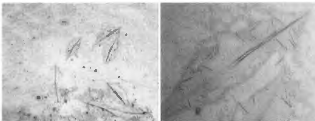
Figure 4-20 Images of the sensor surface with “leaf-like” structures. Magnification \times 2 (left) and magnification \times 10 (right).
