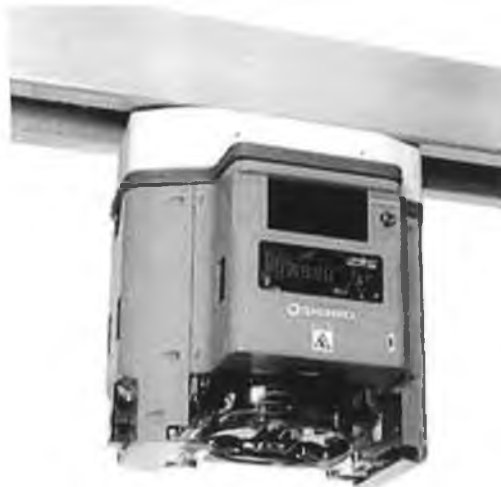
Figure 3.9: Overhead Hoist Vehicle (Courtesy of Shinko Technologies, Inc. [89]).
