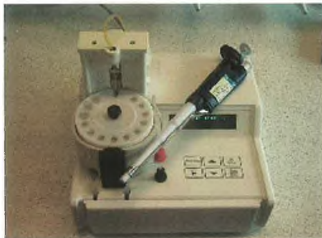
Figure 2.2: Envitec prototype device for rapid analysis of drugs of abuse in saliva samples.
