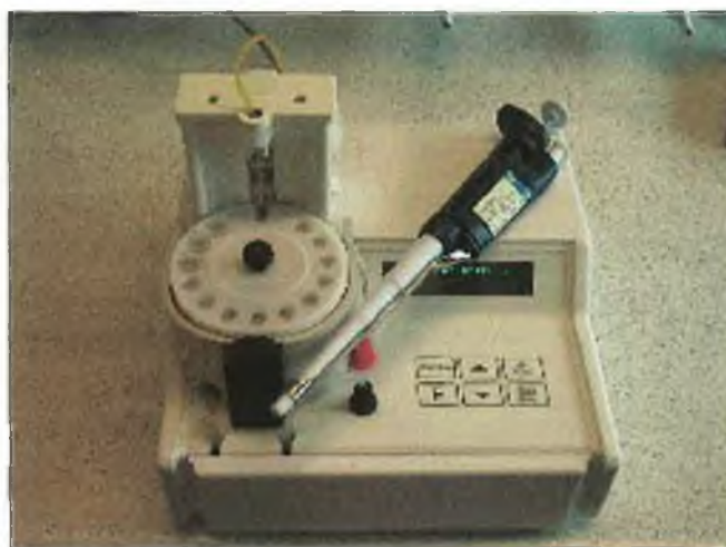
Figure 6.1: Envitec prototype device for rapid analysis of drugs of abuse in saliva samples.
