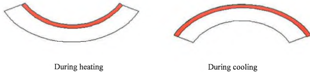
Figure 5.25. Bending of the coating-substrate system after the generation of thermal stress in finite element modelling.
