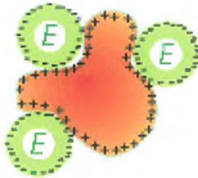
Figure 1.15.4.1: Adsorption of enzymes to an insoluble material. The green circles marked E are the enzymes the red shape is the water insoluble material
