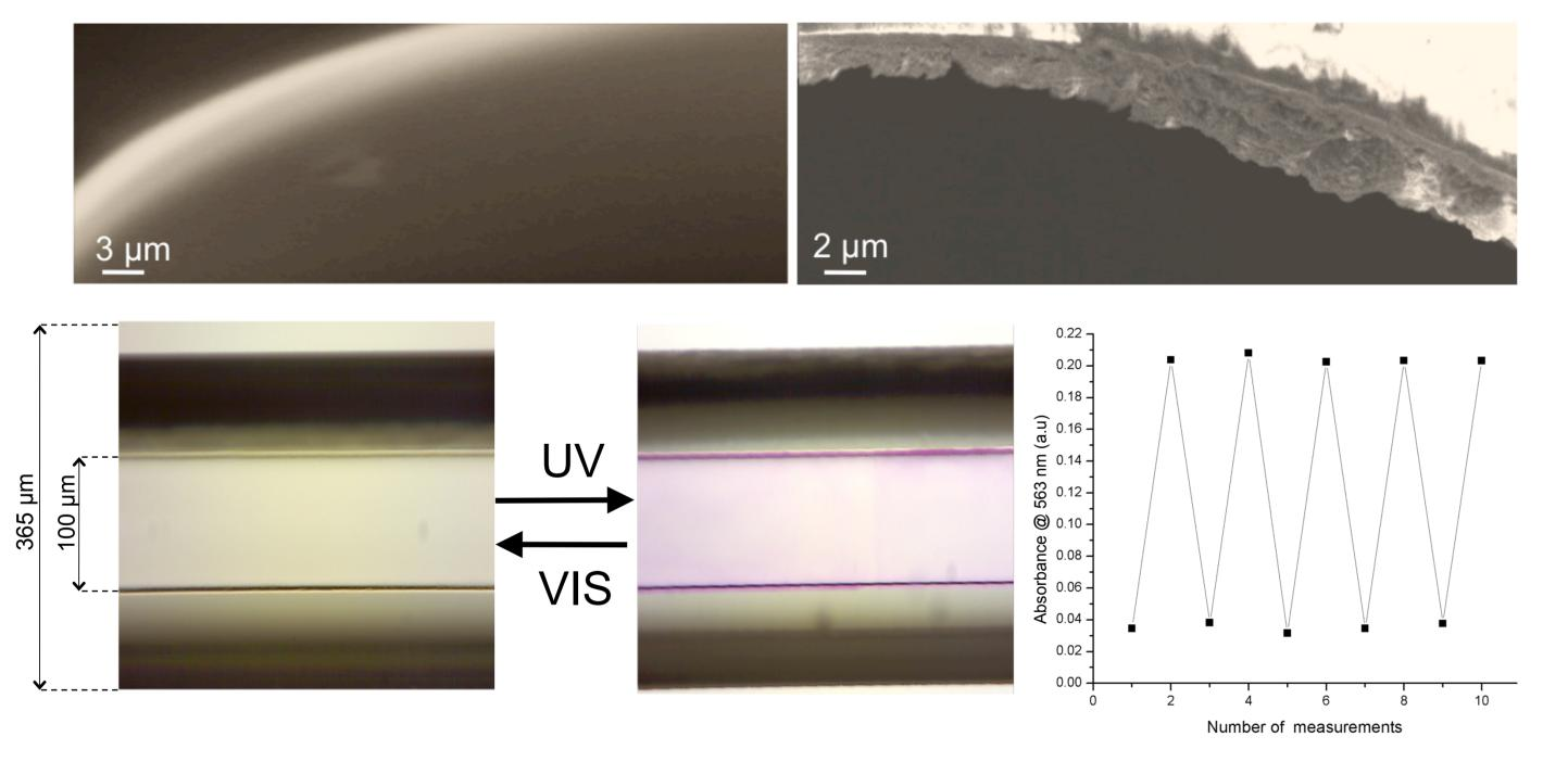
The open MC form exibits particular metal ion binding proprieties - this behaviour is not manifested by the closed spiropyran form. Photoswitchable coatings based on spiropyran can be used to photo-detect divalent metal ions solutions when passing through the capillary.
