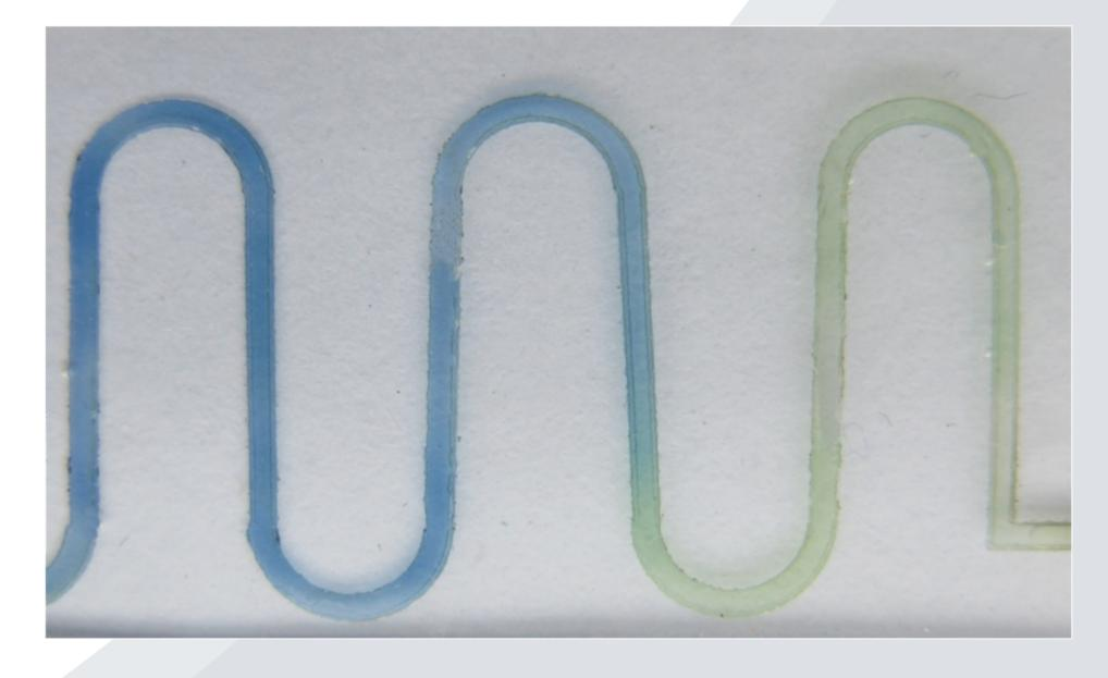
UV-Vis spectra of PAni coatings are measured for each pH solutions that is passed through the channel. Moreover, the PAni coatings have the ability of sensing pH gradients induced in the micro-channel.
